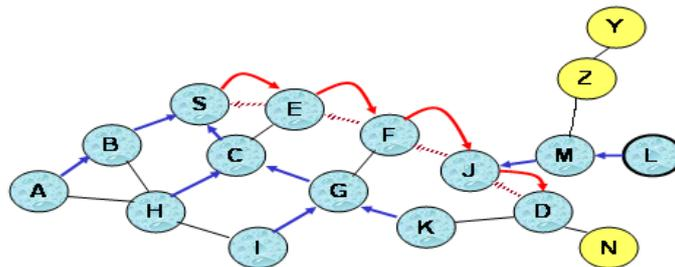
Figure.4. Packet sending from S to D.
