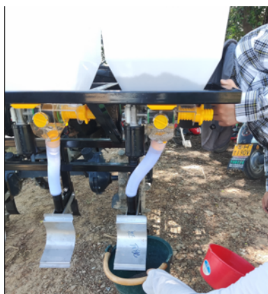
Figure 5. Spiral groove wheel model validation test.
