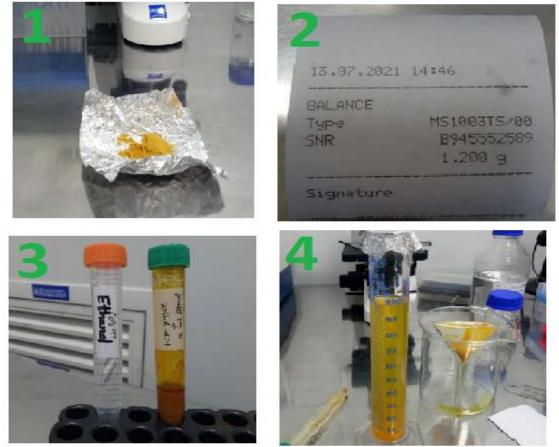
Figure-1: 1&2) 1.2g Ginger power and the record sheet of weight machine during taking weight, 3&4) Dissolve it in Ethanol and filtration after mixing it and resting it 24 hours.
