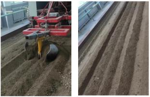
(a) operation process (b) operation effect **Figure no 7 :** In-situ tilling plow test
