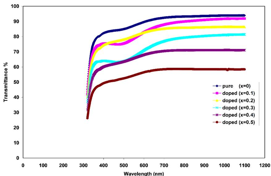
**Figure (1):** transmittance as a function of wavelength for (TiO<sub>2</sub>)<sub>1-x</sub>(Ag)<sub>x</sub> films deposited on glass substrate with different Ag contents.
