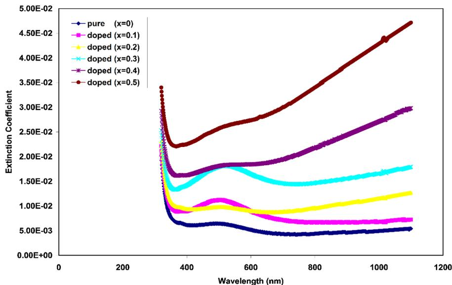
**Fig. (6):** extinction coefficient as a function of wavelength for  $(\text{TiO}_2)_{1-x}(\text{Ag})_x$  films deposited on glass substrate with different Ag content.
