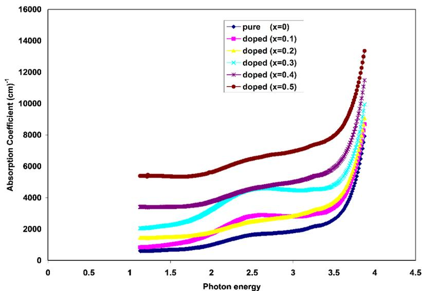
**Figure (3):** Absorption coefficient as a function of photon energy for  $(\text{TiO}_2)_{1-x}(\text{Ag})_x$  films deposited on glass substrate with different Ag contents.
