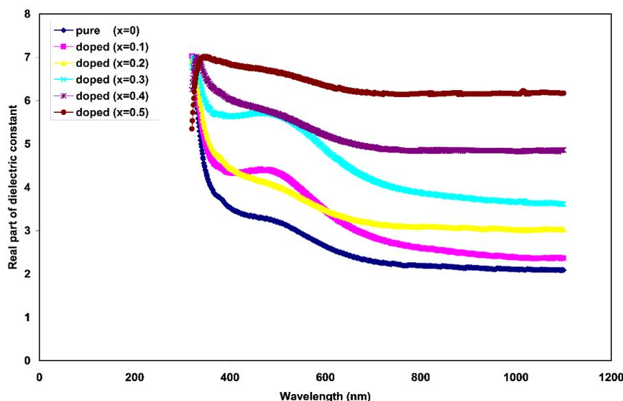
**Fig. (7):** Real ( $\epsilon_r$ ) parts of the dielectric function as a function of wavelength for  $(\text{TiO}_2)_{1-x}(\text{Ag})_x$  films deposited on glass substrate with different Ag contents.
