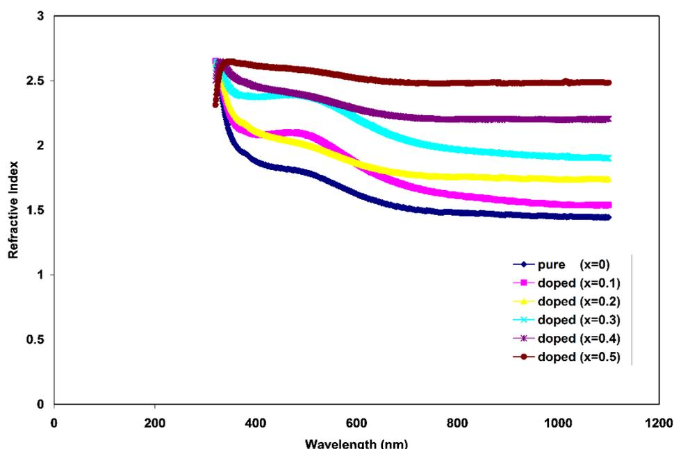
**Fig. (5):** Refractive index as a function of wavelength for  $(TiO_2)_{1-x}(Ag)_x$  films deposited on glass substrate with different Ag content.
