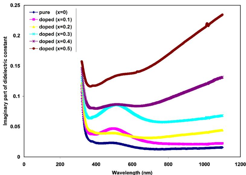
**Fig. (8):** Imaginary ( $\epsilon_i$ ) parts of the dielectric function as a function of wavelength for  $(\text{TiO}_2)_{1-x}(\text{Ag})_x$  films deposited on glass substrate with different Ag content.
