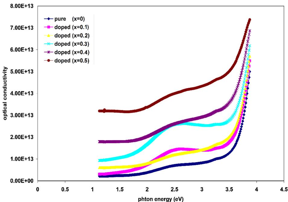
**Fig. (9):** Optical conductivity as a function of photon energy for  $(\text{TiO}_2)_{1-x}(\text{Ag})_x$  films deposited on glass substrate with different Ag contents.
