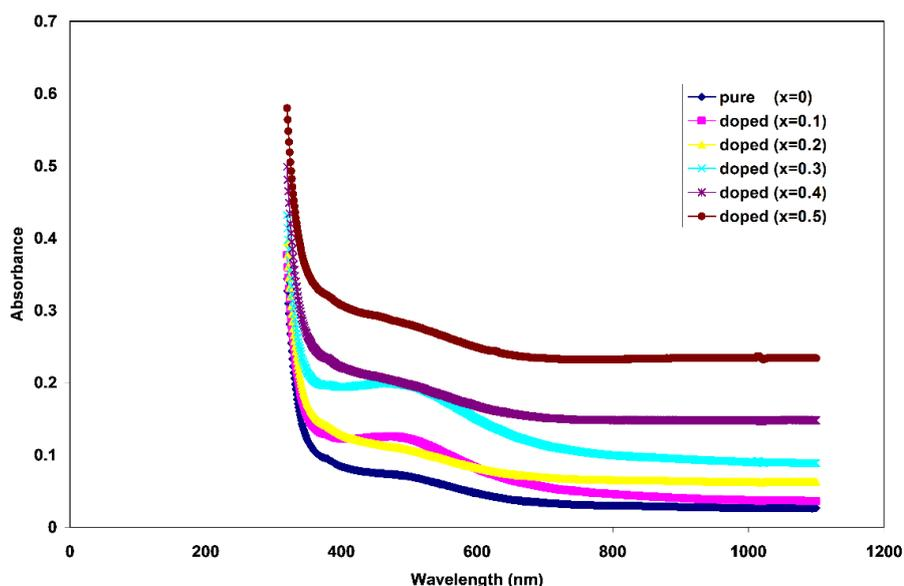
**Fig. (2):** absorbance spectra as a function of wavelength for (TiO<sub>2</sub>)<sub>1-x</sub>(Ag)<sub>x</sub> films deposited on glass substrate with different Ag contents.
