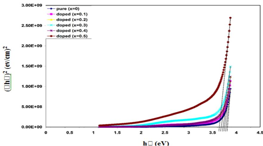
**Fig. (4):** Allowed direct electronic transitions of  $(\text{TiO}_2)_{1-x}(\text{Ag})_x$  films deposited on glass substrate with different Ag contents.
