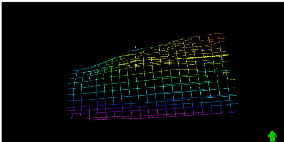
Fig. 8a: Interpreted horizon on reservoir D top
