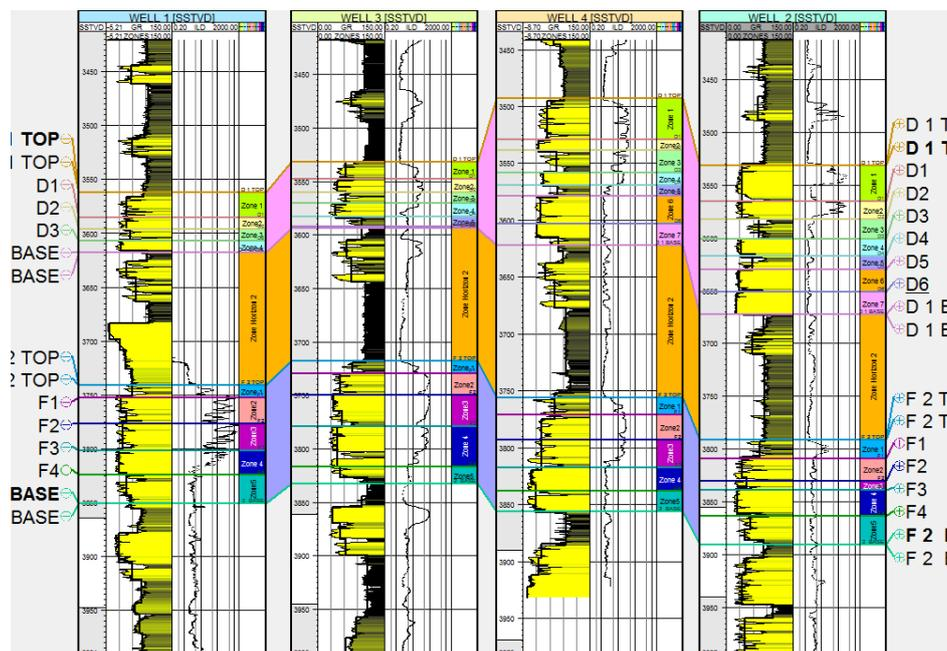
**Fig. 16:** Delineated zones on the well section
