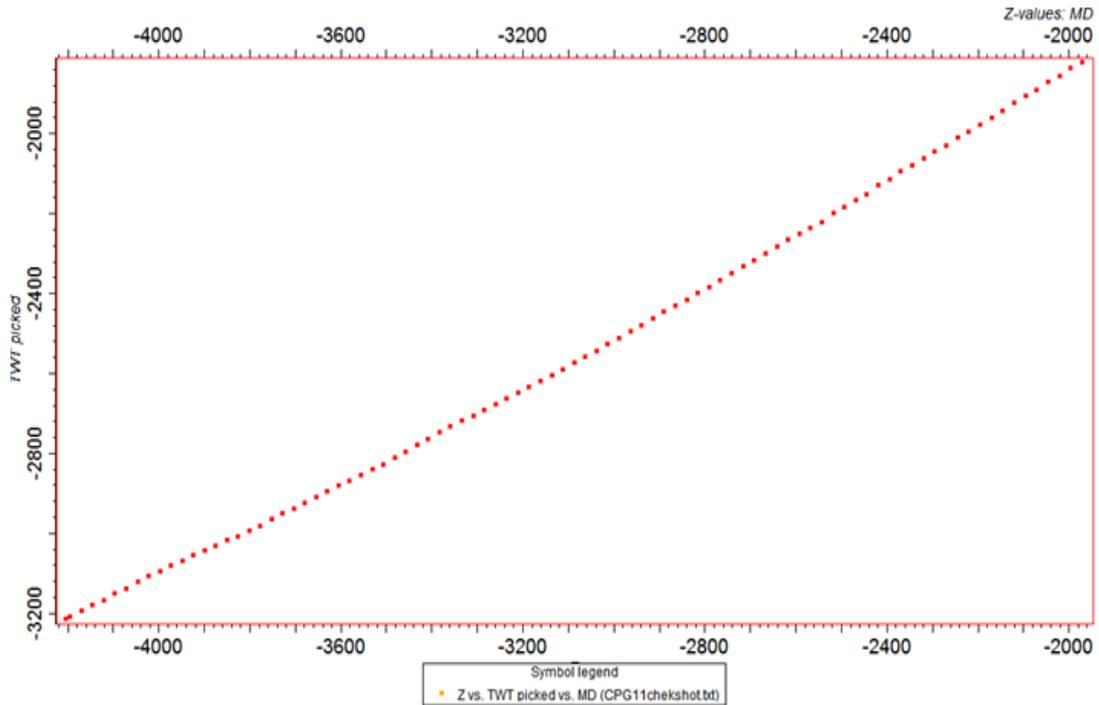
Fig. 5: TWT-Z Curve for D checkshot used for Depth Conversion
