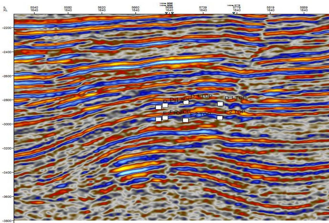
Fig. 4: Well-to-seismic Tie of D and F
