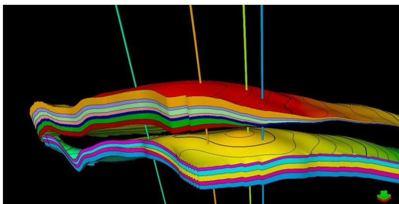
**Fig. 14:** Structural models of reservoirs D and F stalked.
