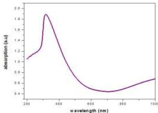
Fig. 4 Wavelength vs Absorbance of Zinc doped CuS thin film
