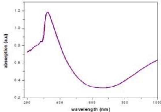
Fig. 3 Wavelength vs Absorbance of CuS thin film.
