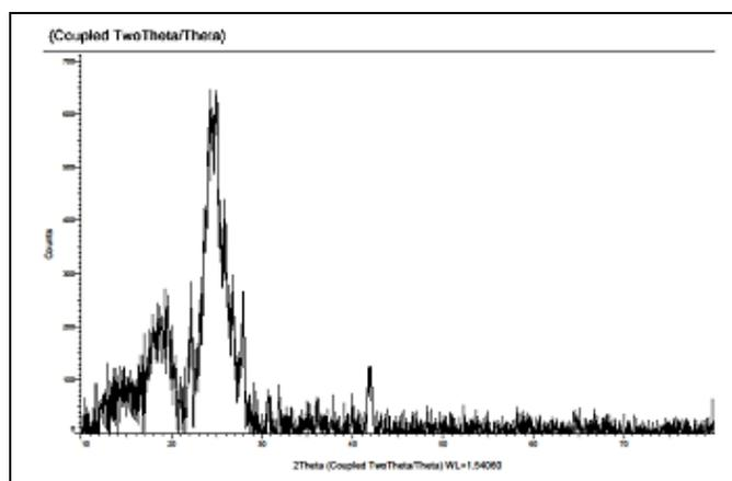
Fig.2. XRD of Pani/ZnS nanocomposite (25%)
