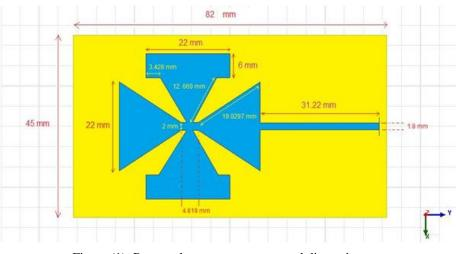
Figure (1): Proposed antenna geometry and dimensions.
