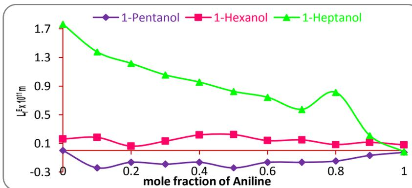
**Fig-5.** Mole fraction vs excess free length at 303k.
