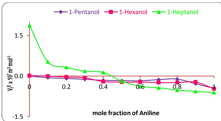
**Fig-6.** Mole fraction vs excess free volume at 303k.
