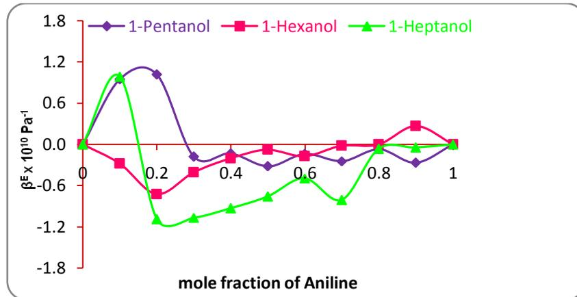
**Fig-4.** Mole fraction vs excess adiabatic compressibility at 303 k.
