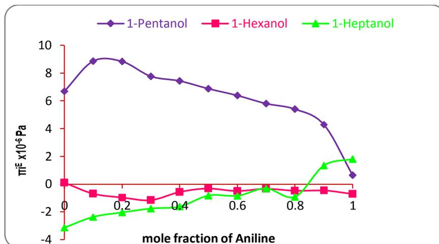
Fig-7. Mole fraction vs excess internal pressure at 303k.
