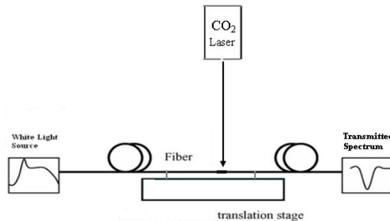
Figure 3. Schematic diagram of fabrication of LPG
