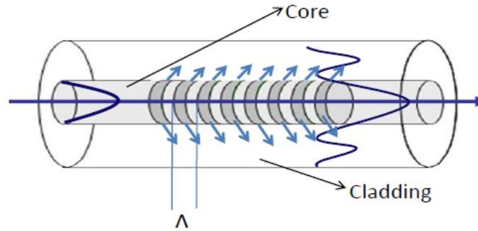
Figure 2. Operating principle of LPG.
