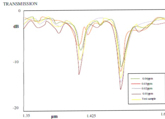
Figure 5. Spectral behavior of LPFG for manganese solution of different concentrations.
