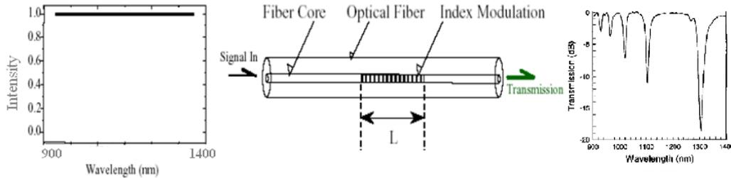
Figure 1. Transmission spectrum of input signal through LPFG.
