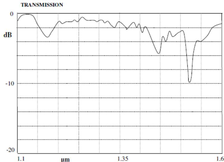
Fig. 4. Transmission spectrum of fabricated LPG
