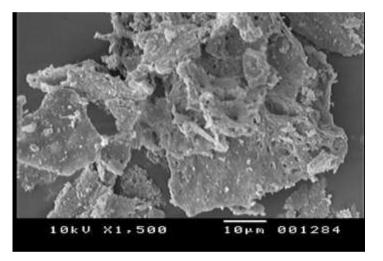
Fig-3(b) SEM Morphology of Sintered  $Ni_{0.2}CO_{0.5}Zn_{0.3}Fe_2O_4$  Ferrites.
