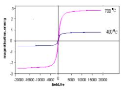
Fig.4 (a): Hysteresis loops of  $Ni_{0.2}Co_{0.2}Zn_{0.6}$  sintered at 400°C and 700°C
