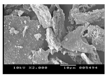
$\label{eq:Fig-3(c)} \begin{array}{l} \mbox{Fig-3(c) SEM Morphology of Sintered} \\ Ni_{0.2}CO_{0.2}Zn_{0.6}Fe_2O_4 \mbox{ Ferrites} \end{array}$
