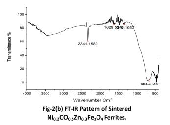
The of  $Ni_{0.2}CO_{0.5}Zn_{0.3}Fe_2O_4$  IR curve fig2(b) of sintered powder shows strong absorption band 1345.10Cm<sup>-1</sup> to 1629.55Cm<sup>-1</sup> indicates N-H Bending structure, the strong absorption band at 2341.15Cm<sup>-1</sup> indicating C triple bond N- Stretched. The band at 668.21 Cm<sup>-1</sup> indicating C-H out of plane bending carbohydrates which is very weak and shifted to low frequency.
