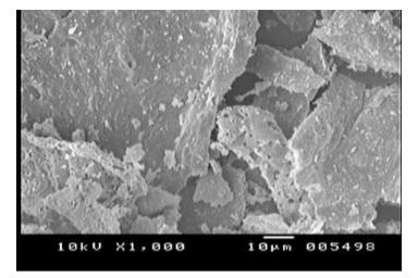
Fig-3(a)SEM Morphology of Sintered Ni<sub>0.2</sub>CO<sub>0.2</sub>Zn<sub>0.6</sub>Fe<sub>2</sub>O<sub>4</sub> Ferrites.
