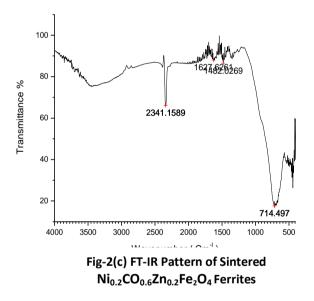
The of  $Ni_{0.2}CO_{0.6}Zn_{0.2}Fe_2O_4$  IR curve fig2(c) of sintered powder shows strong absorption band 14825.027Cm<sup>-1</sup> to 1627.62Cm<sup>-1</sup> indicates N-H Bending structure, the strong absorption band at 2341.15Cm<sup>-1</sup> indicating C triple bond N- Stretched. The band at 714.49 Cm<sup>-1</sup> indicating C-H out of plane bending carbohydrates which is very weak and shifted to low frequency.
