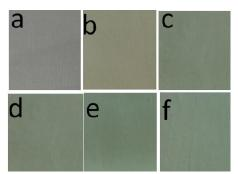
Fig 1 . Digital images of matrix (a), NCCFs made using 1 mM (b), 5 mM (c), 25 mM (d), 125 mM (e) and 250 mM (f) source solutions
