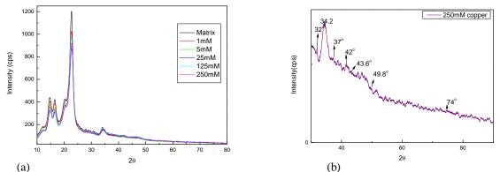
Fig. 2 X-ray diffractograms of the matrix and the NCCFs with in situ generated CuNPs using 1 mM, 5 mM, 25 mM, 125 mM and 250 mM source solutions (a) and Expanded diffractogram of the NCCF with in situ generated CuNPs using 250 mM source solution in  $2\theta$ = 35° to 80° (b).
