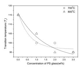
Fig.4: Variation of transition temperature  $(T_c)$  Vs concentration of PS glass (1 to 3wt %) at 700 and  $800^{\circ}$ C sintered temperature
