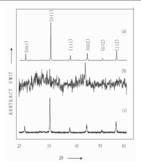
Fig.1: XRD patterns of (a) PFN (b) 4PbO:SiO<sub>2</sub> glass and (c) 0.99{PFN}-0.1{4PbO: SiO<sub>2</sub>}
