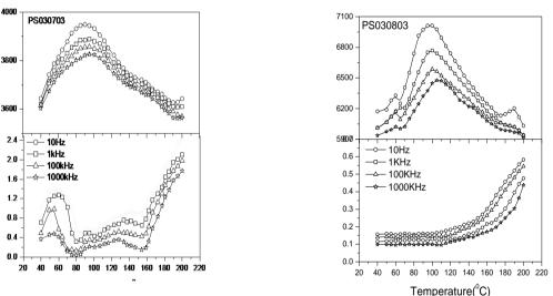
Fig.3: Dielectric constant and dielectric loss of sample (a) F7G3 and (b)F8G3
