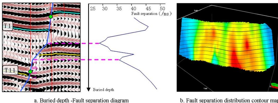
Figure.1 Analysis of well seismic data and break distance of break point
