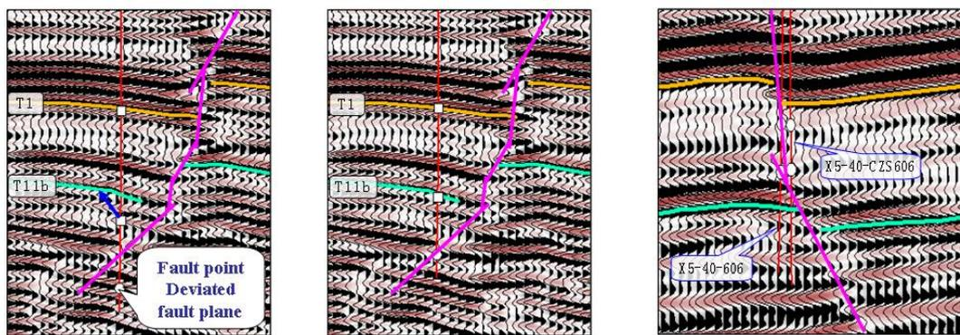
a. Well seismic calibration error b. Corrected well seismic correspondence c. Deviation data error and fault plane does not match the breakpoint
