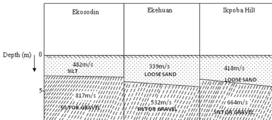
Figure 5: Summary of the seismic refraction survey results for the three locations
