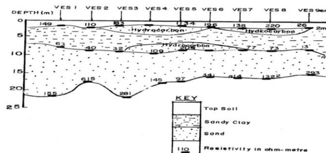
Figure 3 Subsurface soil profile of the spill site from VES data
