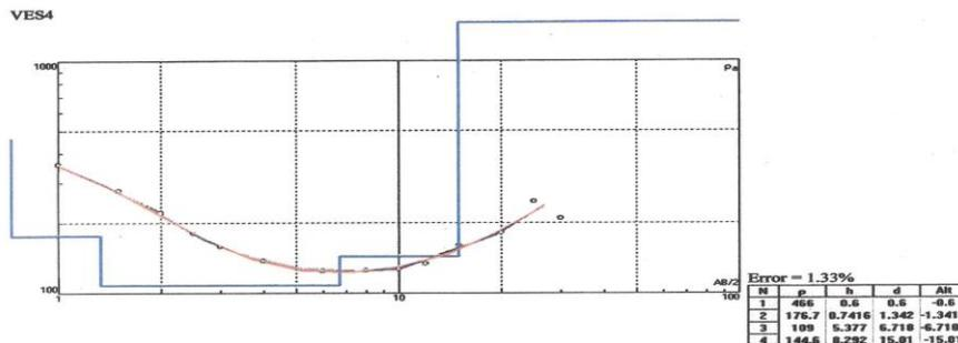
Fig. 2c: Resistivity curve of VES 4
