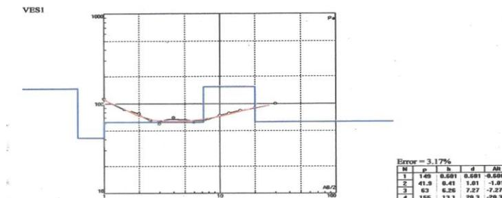
Fig. 2a: Resistivity curve of VES 1
