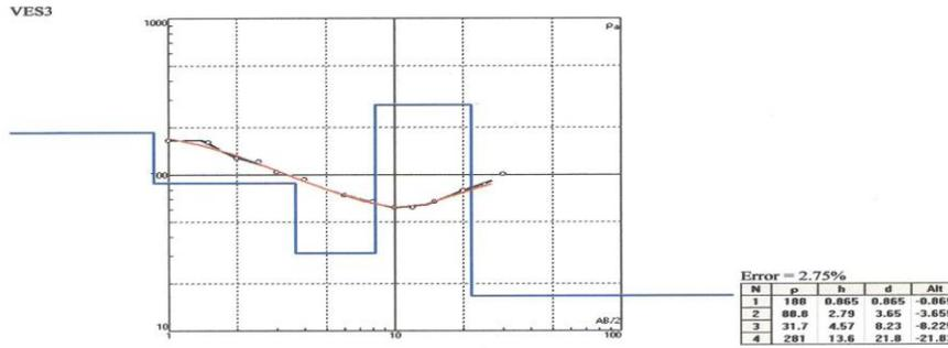
Fig. 2b: Resistivity curve of VES 3
