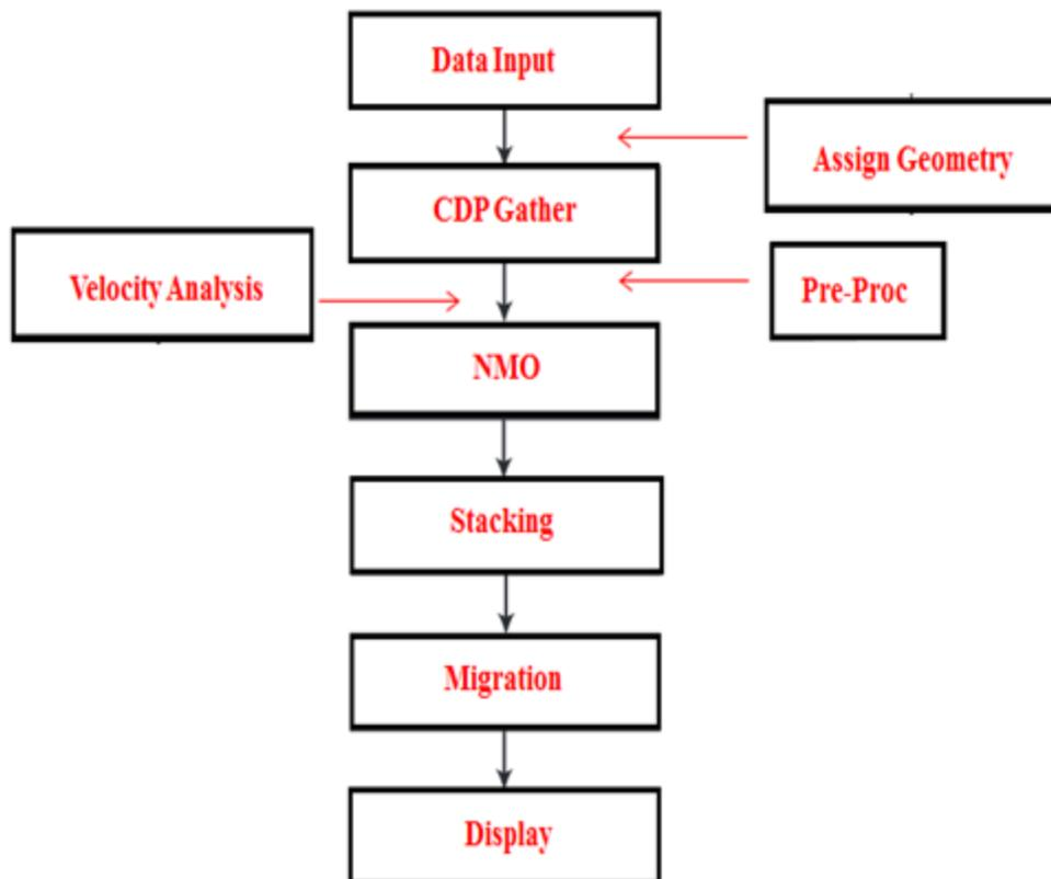
**Figure 4.** Basic processing flow used in this experiment
