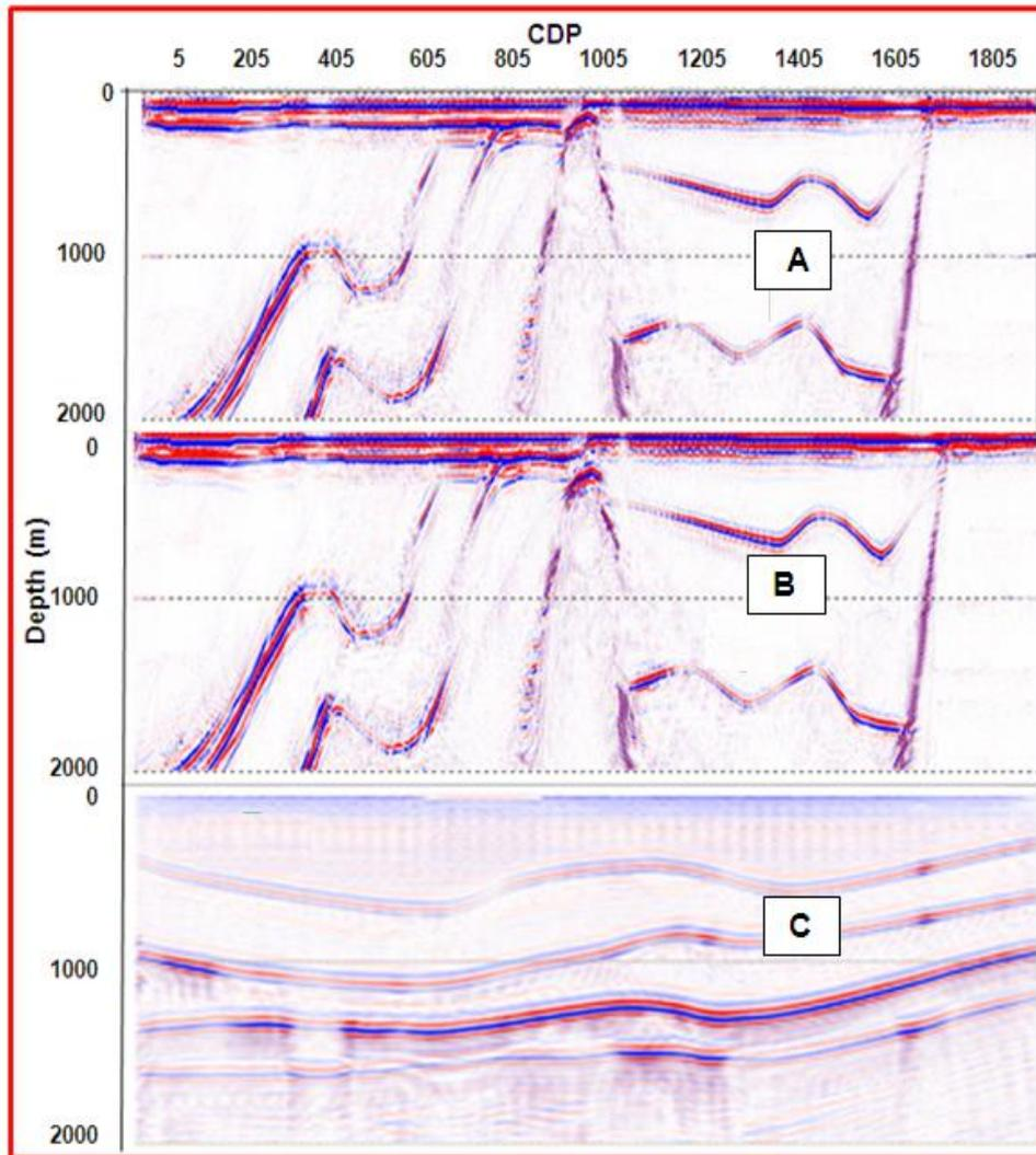
**Figure 5:** Migrated section: Panels (a), and (b) show the effect of different survey parameters in imaging the intrusive near the fault boundary (tight vs sparse). Panels (c) is the migrated section of non intrusive structure (only metasediments). In panels (a) and (b), the top of the intrusive can be detected near the fault.
