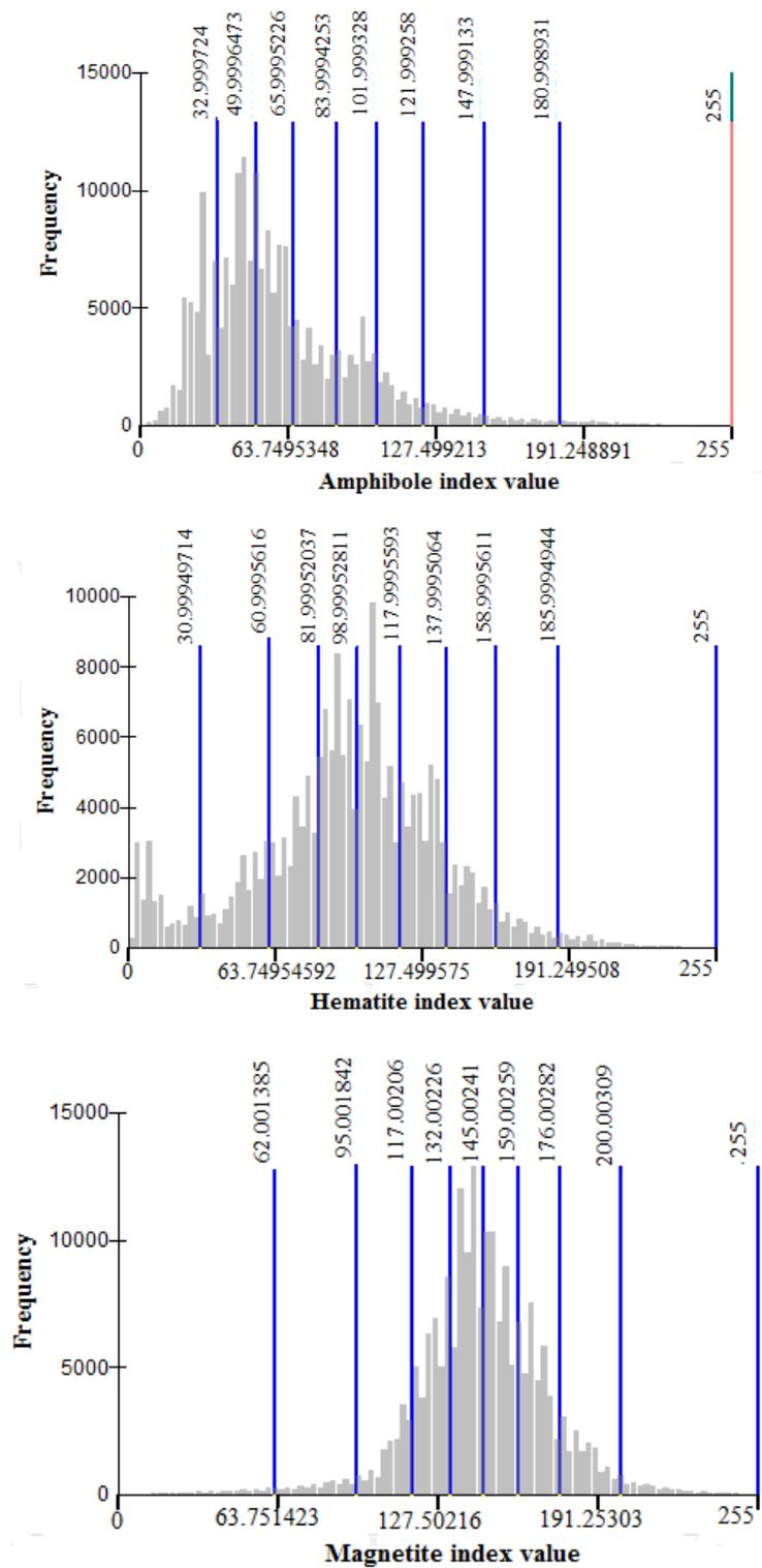
Figure 3. Histograms of Amphibole, Hematite, and Magnetite index maps.
