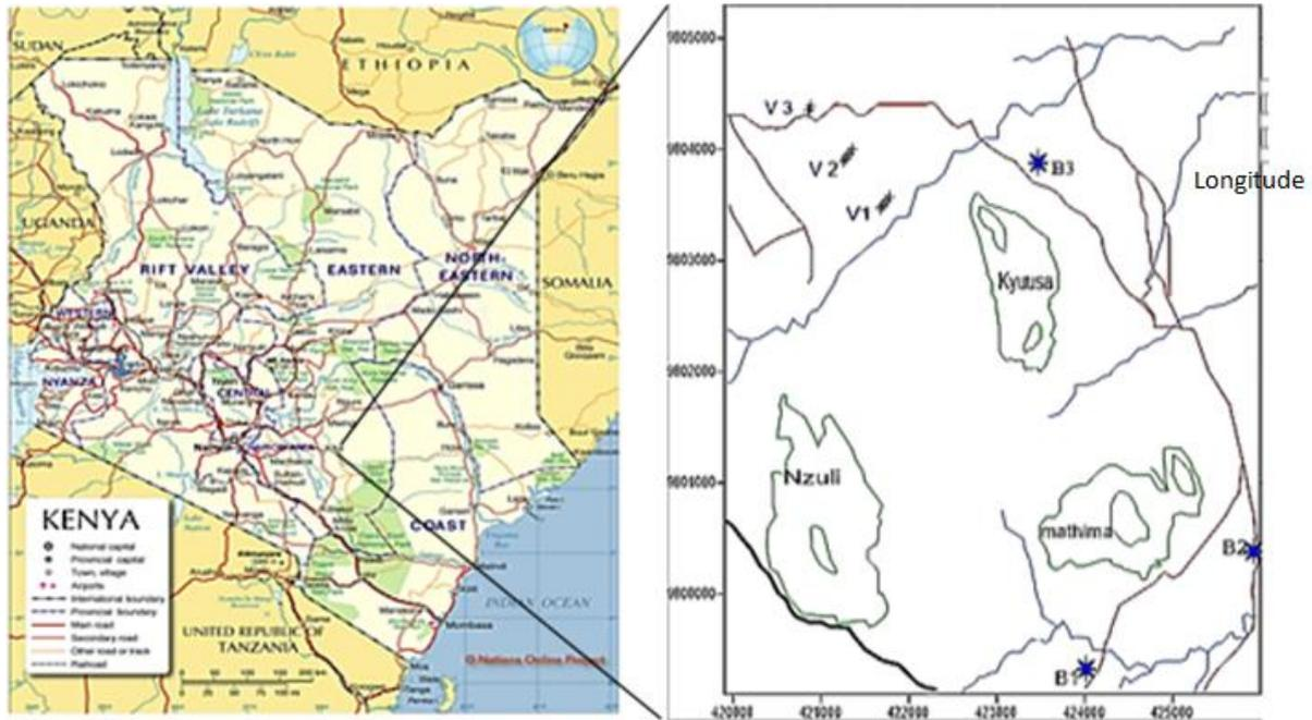
**Figure 1.** A map of the area of study showing the drainage, VES stations and boreholes within area of study. (Note B1, B2 and B3 are boreholes in the area of study, V1, V2 and V3 represent the VES stations)
