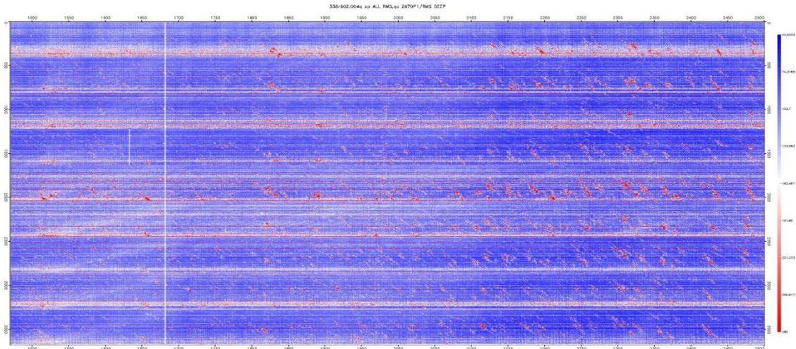
Fig. 3a: RMS window INPUT before swell noise attenuation.
