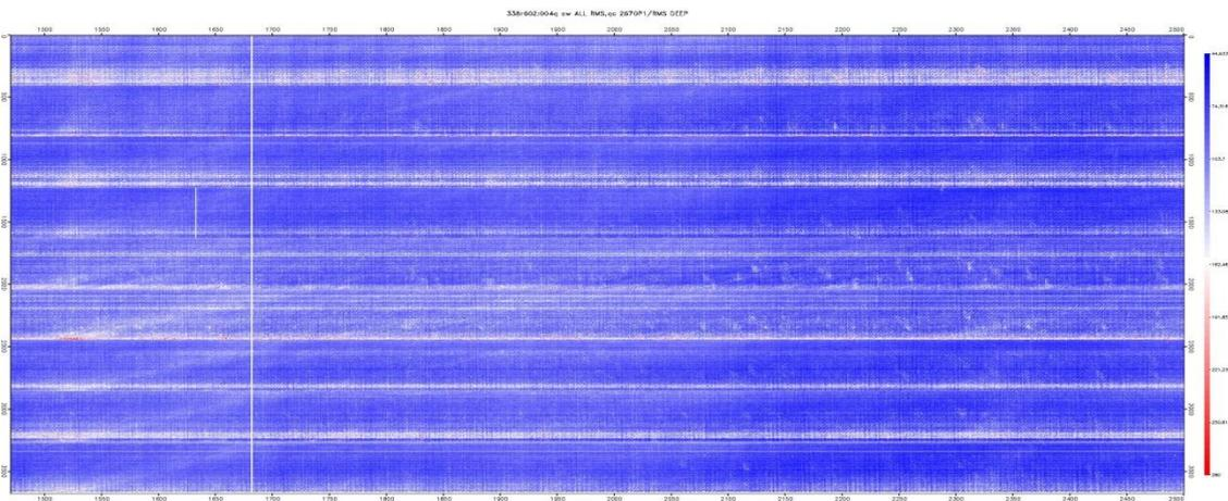
Fig. 3b: RMS window OUTPUT after swell noise attenuation.
