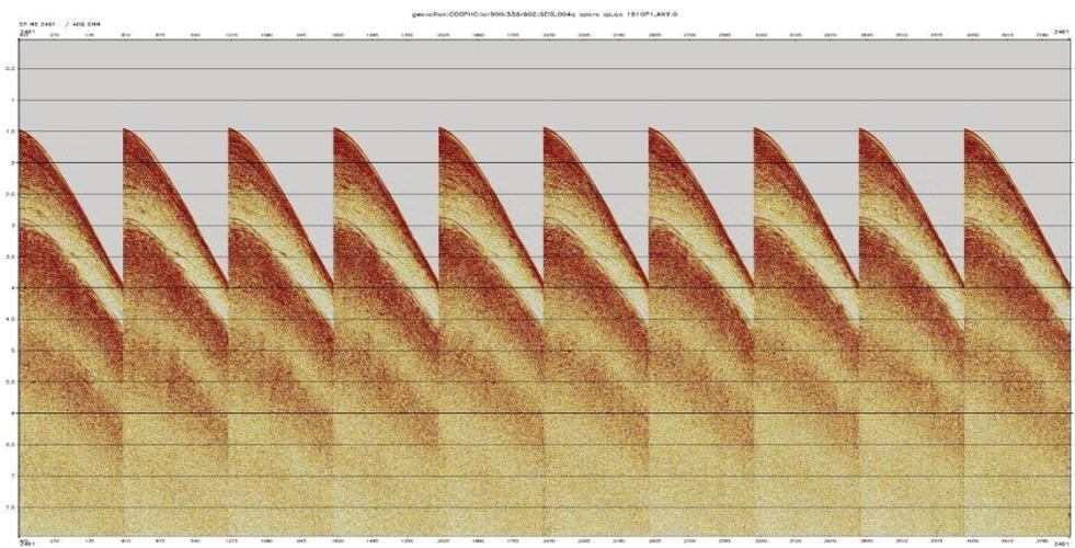
Fig. 1b: Data after application of swell noise attenuation processes
