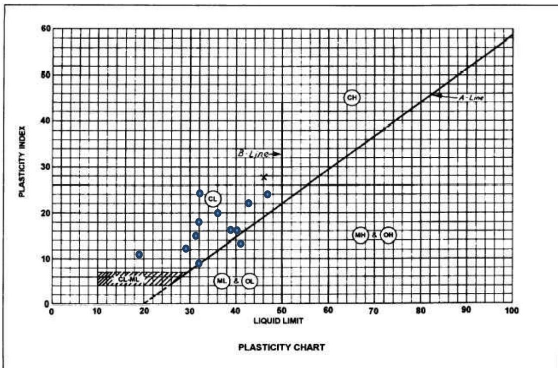
**Figure 3:** Casagrande (1948) plasticity chart showing relative positions of samples
