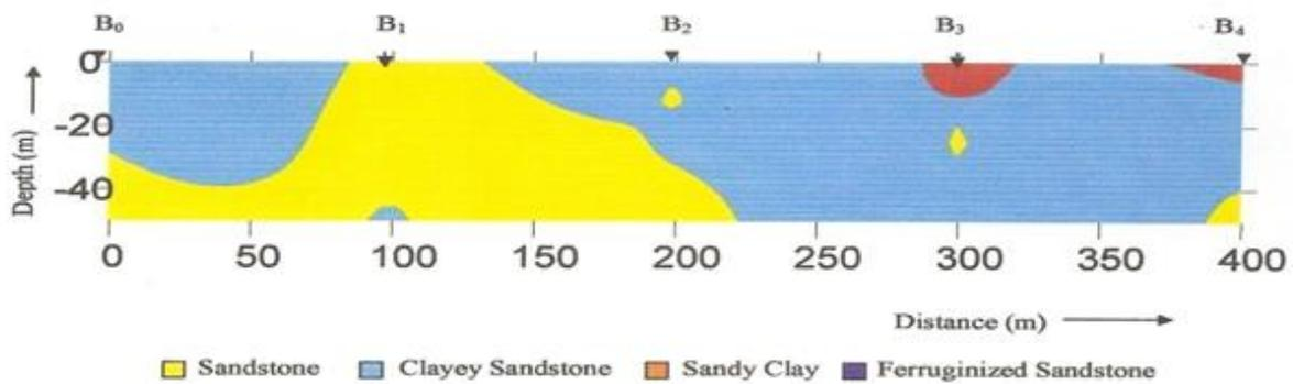
Fig. 3: Geologic Section of Profile B
