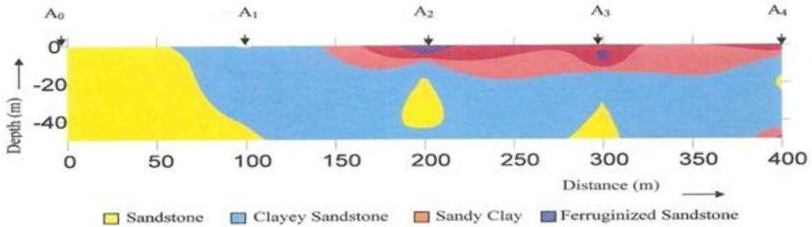
Fig. 2: Geologic Section of Profile A
