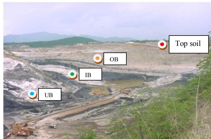
Figure 3 Looking NW on the opening mine face, clay layers of the mine classified to 3 units: OB (overburden), IB (interburden) and UB (underburden)(source: MRD-ECC, 2001).
