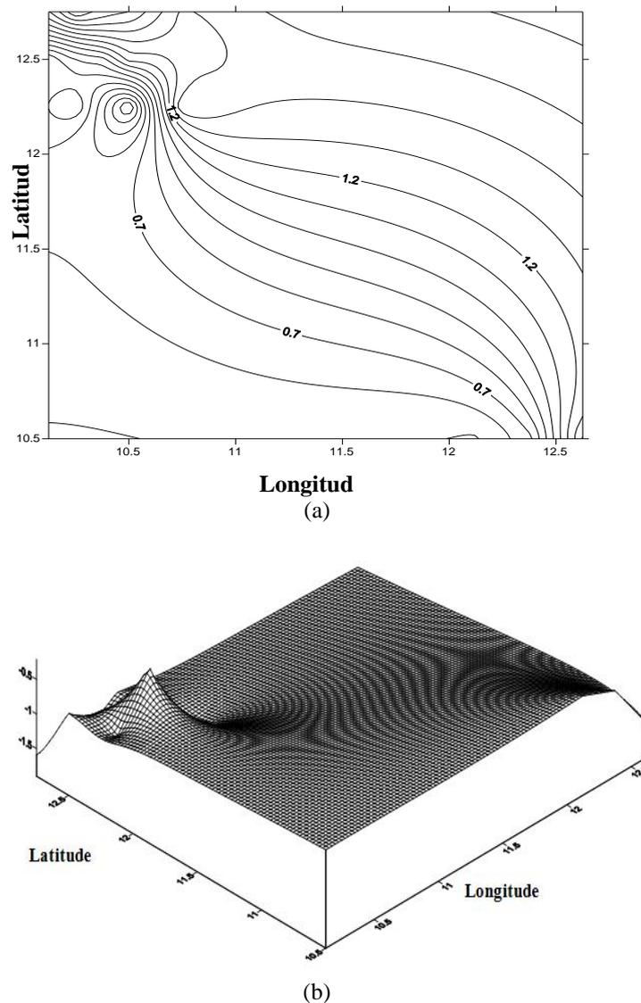
**Figure 4:** (a) Contour map of 1<sup>st</sup> layer magnetic source. (b) Surface map of shallow magnetic source depth.
