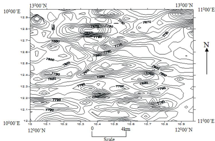
**Figure 2:** Total magnetic intensity map of the study area (contour interval ~ 20nT).
