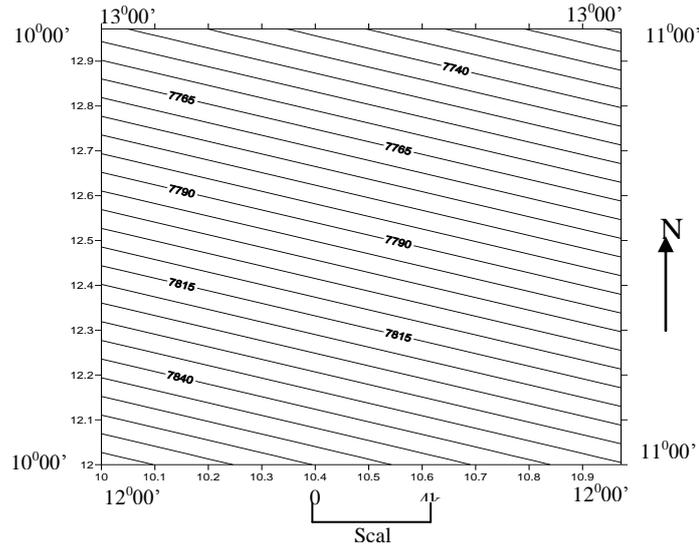
**Figure 3:** Residual anomaly map of the study area (contour interval ~ 20nT).
