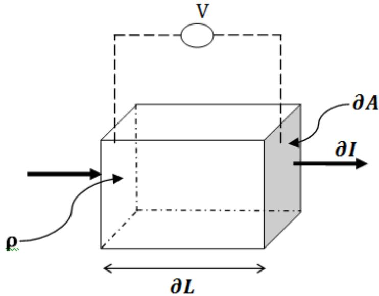
Figure 1: The basic definition of resistivity in a homogeneous block
