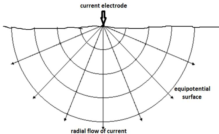
Figure 2.0: The current flowing from electrode to distribute current uniformly over the shell
