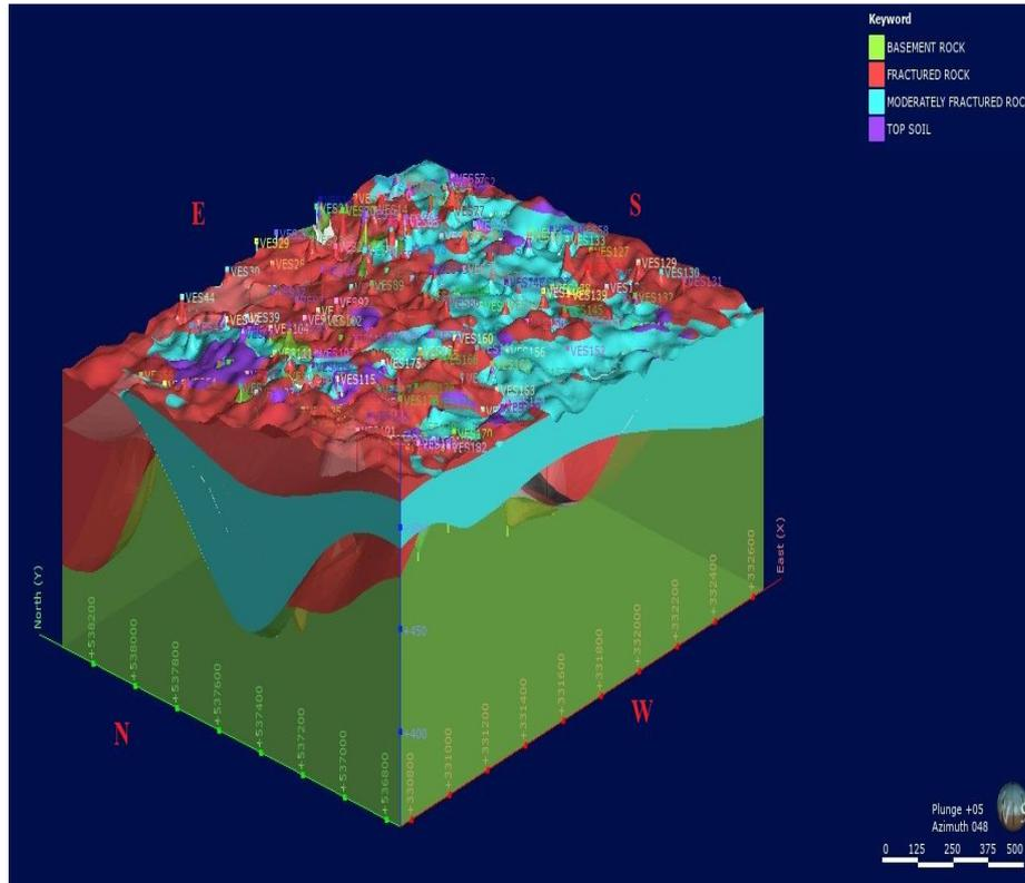
Figure 9: 3D Resistivity models showing North face of Kapuri Area
