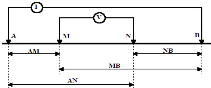
**Figure 4: The generalized form of the electrode configuration used in resistivity measurements**
