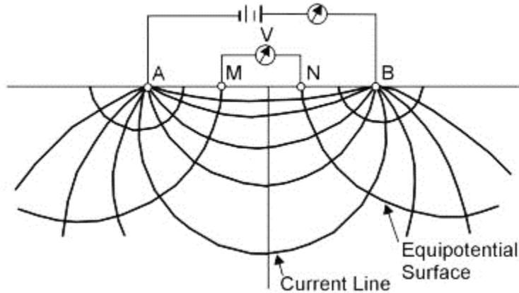
**Figure 3: The potential distribution from a pair of current electrodes (U. S. Environmental Protection Agency, 2011)**
