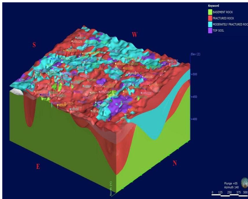
Figure 10: 3D Resistivity models showing south face Kapuri Area
