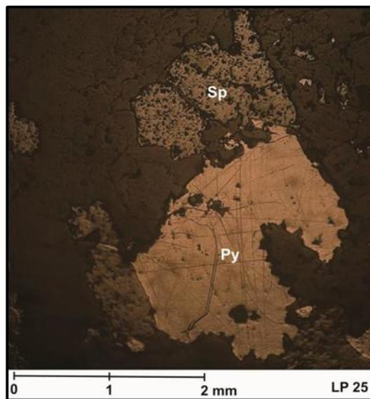
Figure 15. Mineragraphy analysis of sample LP 25 shows pyrite (Py) and sphalerite (Sp) mineral
