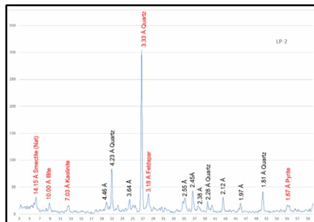
Figure7. The result of XRD analysis at LP 2 shows Smectite, Illite, Kaolinite, Quartz, Pyrite, and Feldspar.
