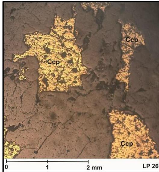
Figure 14. Mineragraphy analysis of the sample from LP 26 shows the presence of chalcopyrite (Ccp) mineral in size up to 2 mm
