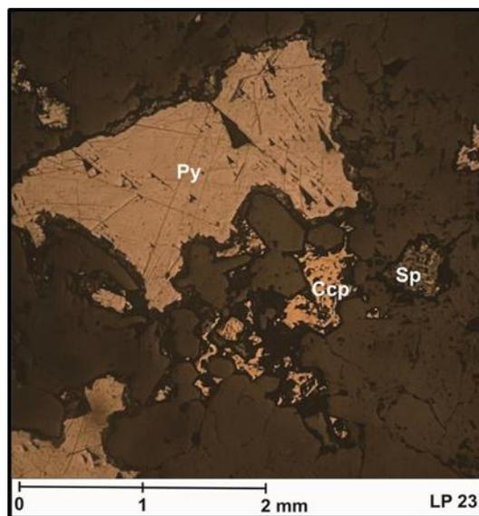
Figure13. Mineragraphy analysis of the sample at LP 23 shows chalcopyrite (Ccp) and pyrite (Py) mineral is substituted by sphalerite (Sp) mineral
