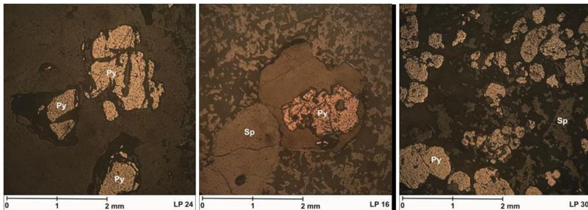
Figure 11. Mineragraphy analysis of the samples at LP 24 (left), LP 16 (middle), and LP 30 (right) shows the presence of pyrite (Py) and sphalerite (Sp) mineral
