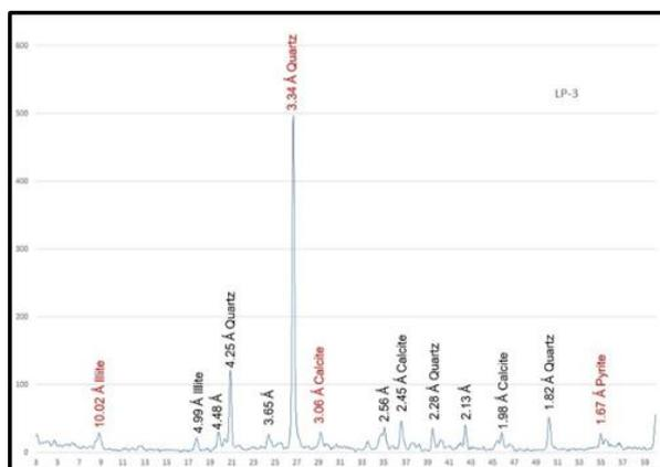
Figure 4. The XRD analysis result at LP 3 shows the presence of Quartz, Illite, Calcite, and Pyrite
