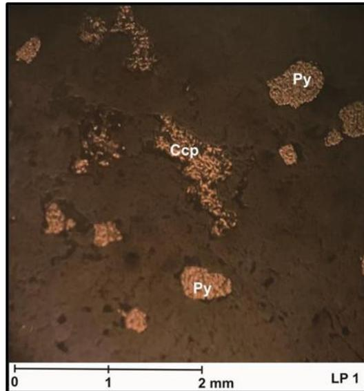
Figure12. The mineragraphy analysis of the sample from LP 1 shows Chalcopyrite (Cp) and Pyrite (Py) mineral
