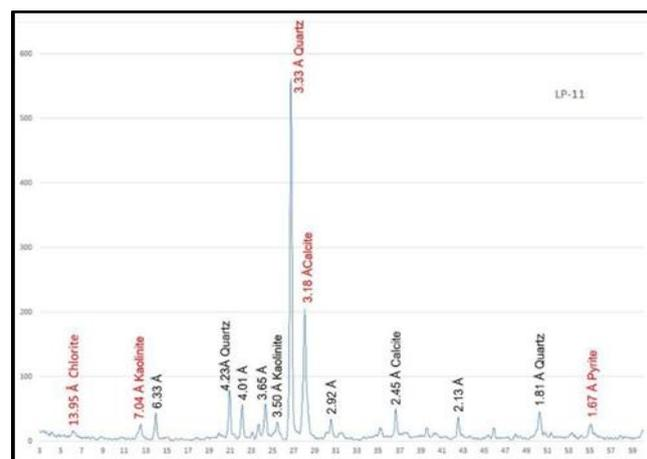
Figure9. The result of XRD analysis at LP 11 shows Chlorite, Kaolin, Calcite, Quartz, and Pyrite
