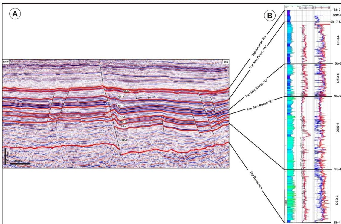
**(Fig. 11):** The integration between the seismic (A) and well (B) datasets showing the subdivision of the Upper Cretaceous megasequence into its depositional sequences (DSQ-3 to DSQ-8) in EON.
