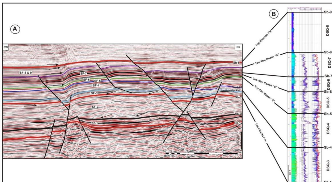
**(Fig. 10):** The integration between the seismic (A) and well (B) datasets showing the subdivision of the Upper Cretaceous megasequence into its depositional sequences (DSQ-3 to DSQ-8) in the WON.
