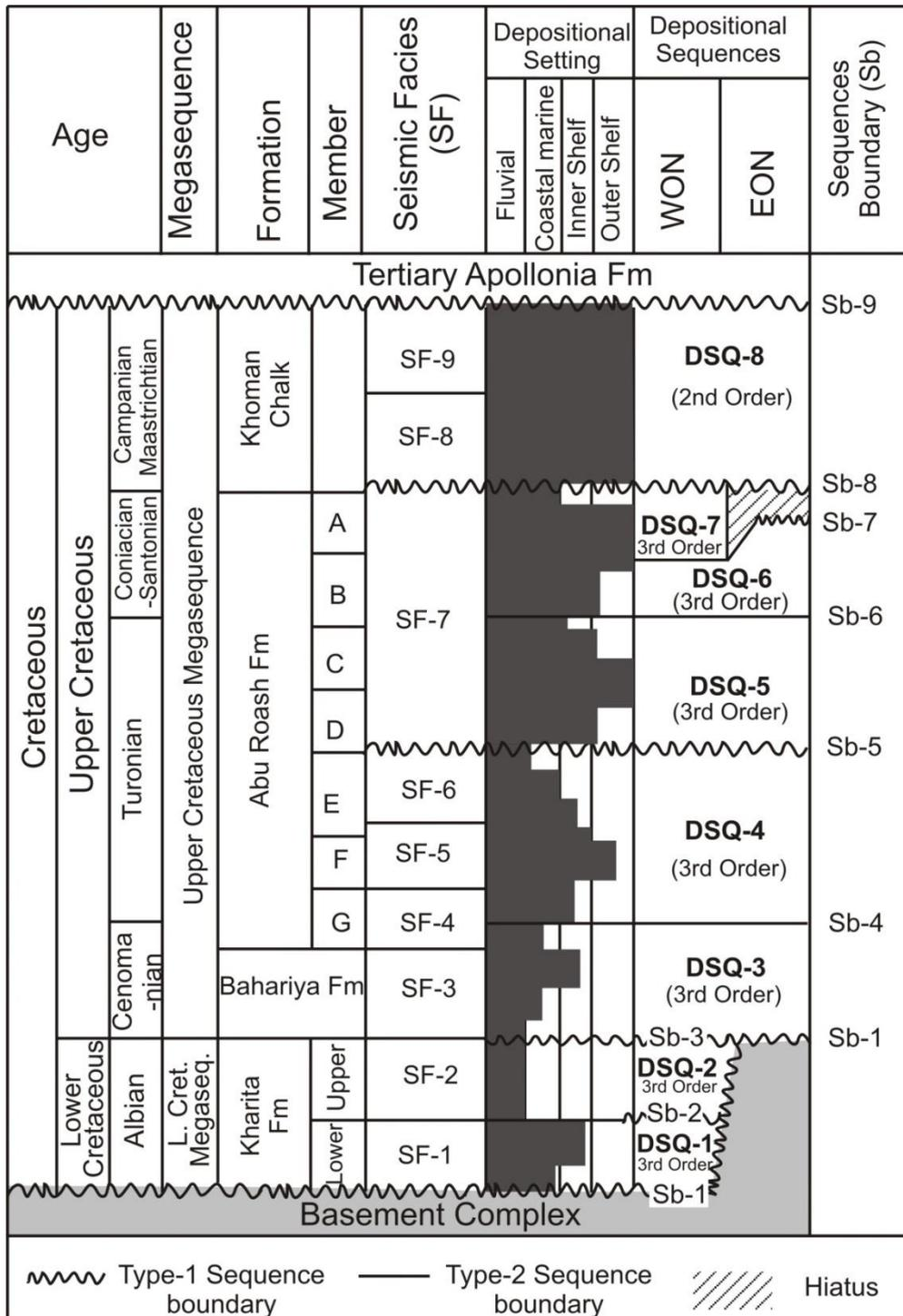
(Fig. 8): The depositional setting and correlation between the encountered Cretaceous seismic facies, depositional sequences and their boundaries on the both sides of the Beni Suef Basin.
