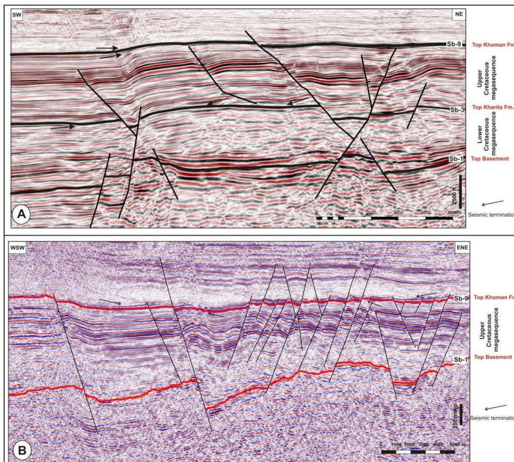
(Fig. 4): NE-SW and WSW-ENE seismic lines showing (A) the Lower and Upper Cretaceous megasequences in the WON, (B) the Upper Cretaceous megasequence in the EON. Notice the seismic terminations (Black arrows). For location see (Figs. 2C and D).
