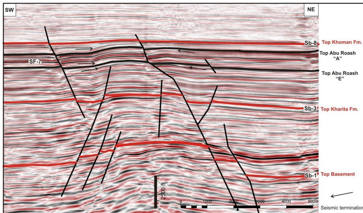
(Fig. 7): NE–SW seismic inline showing the seismic facies 7 (SF-7). Notice the seismic terminations (Black arrows). For location see (Fig. 2C).
