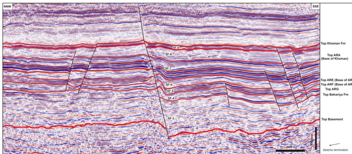
**(Fig. 6):** NW–SE seismic line showing the seismic facies 3 to 9 (SF-3 to SF-9). For location see (Fig. 2D).
