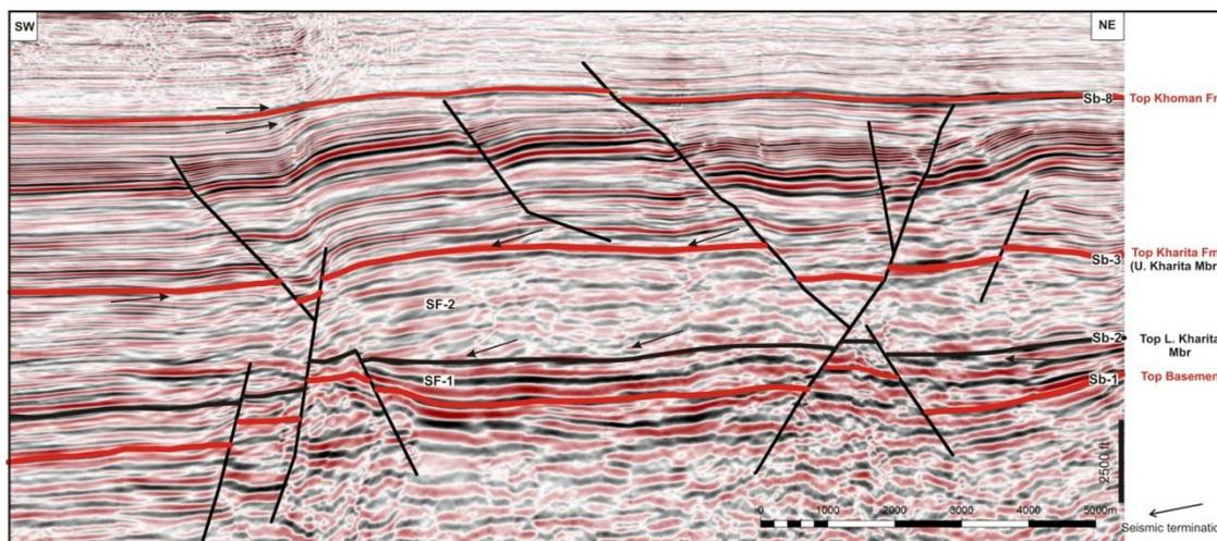
**Fig. 5):** NE–SW seismic line showing the seismic facies (SF-1 & SF-2) in the Lower Cretaceous Megasequence. Notice the seismic terminations (Black arrows). For location see (Fig. 2C).
