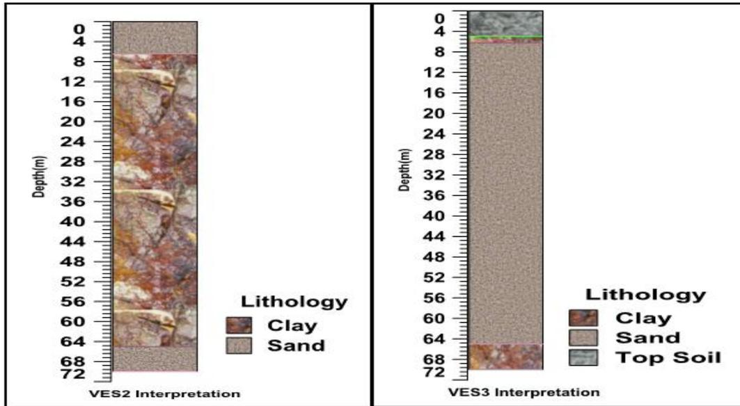
Figure 5: 1-D Geologic section of the subsurface for VES profile 2. Showing a Confined aquifer within the third layer sand unit
