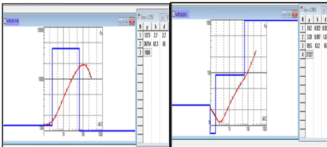
Figure 4 (T): Geo-electric model & layer parameters for VES 20 (HA curve type). Figure 4 (S): Geo-electric model & layer parameters for VES 19 (K type curve).
