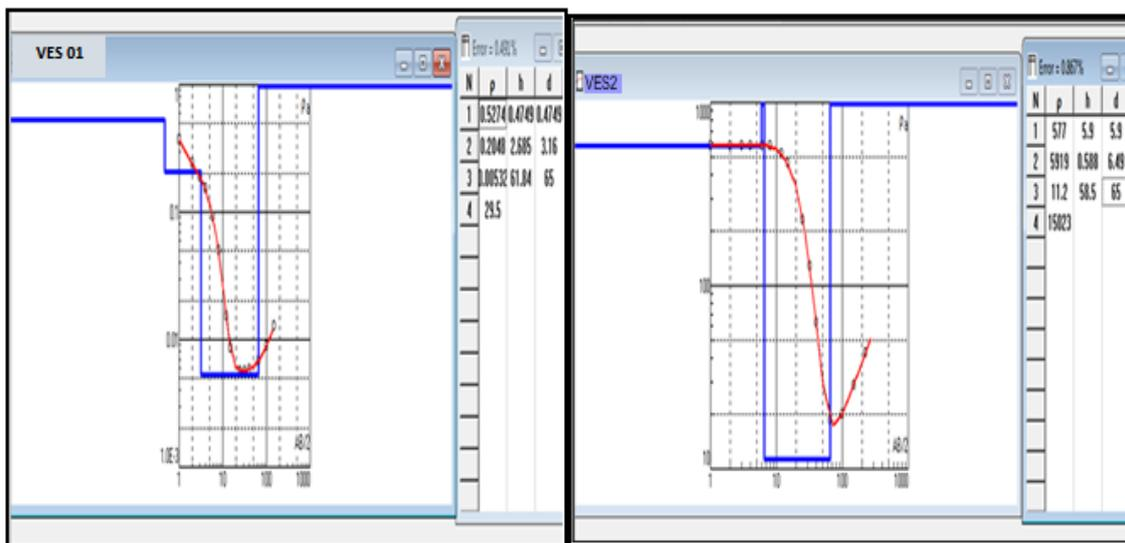
Figure 4 (B): Geo-electric model & layer parameters for VES 2 (KH curve type). Figure 4 (A): Geo-electric model & layer parameters for VES 1 (QH curve type).
