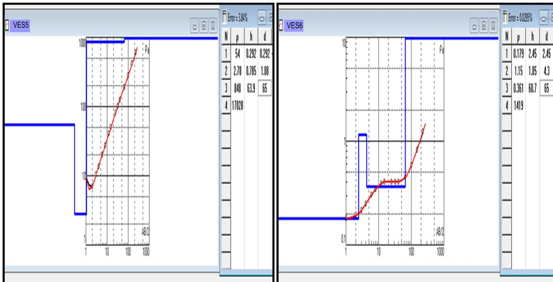
Figure 4 (F): Geo-electric model &layer parameters for VES 6(KH curve type).Figure 4 (E): Geo-electric model &layer parameters for VES 5 (HA curve type).
