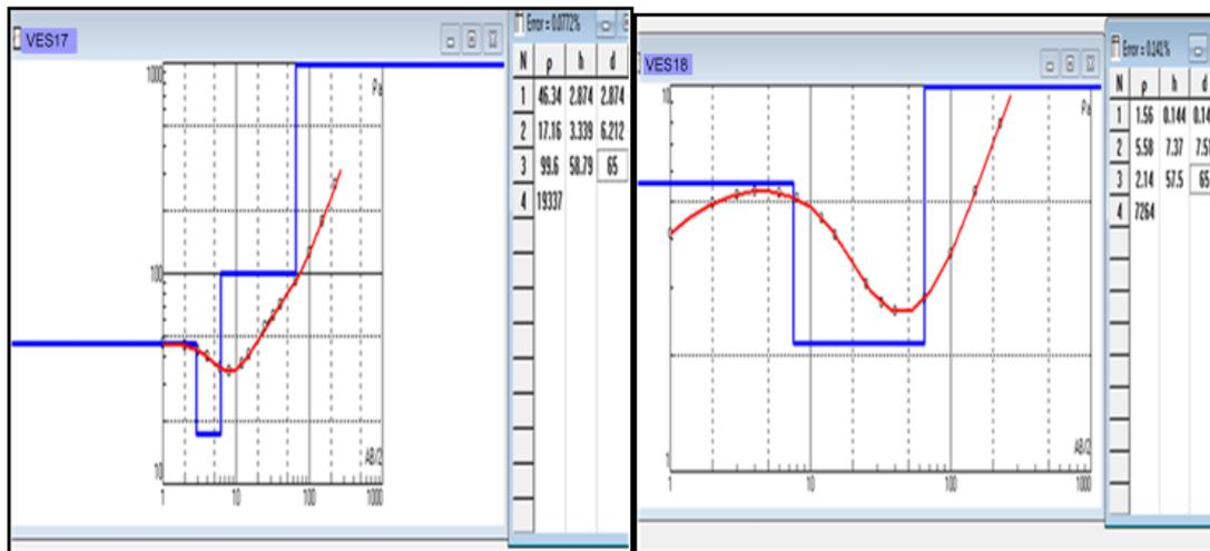
Figure 4 (R): Geo-electric model & layer parameters for VES 18 (KH curve type). Figure 4 (Q): Geo-electric model & layer parameters for VES 17 (HA curve type)
