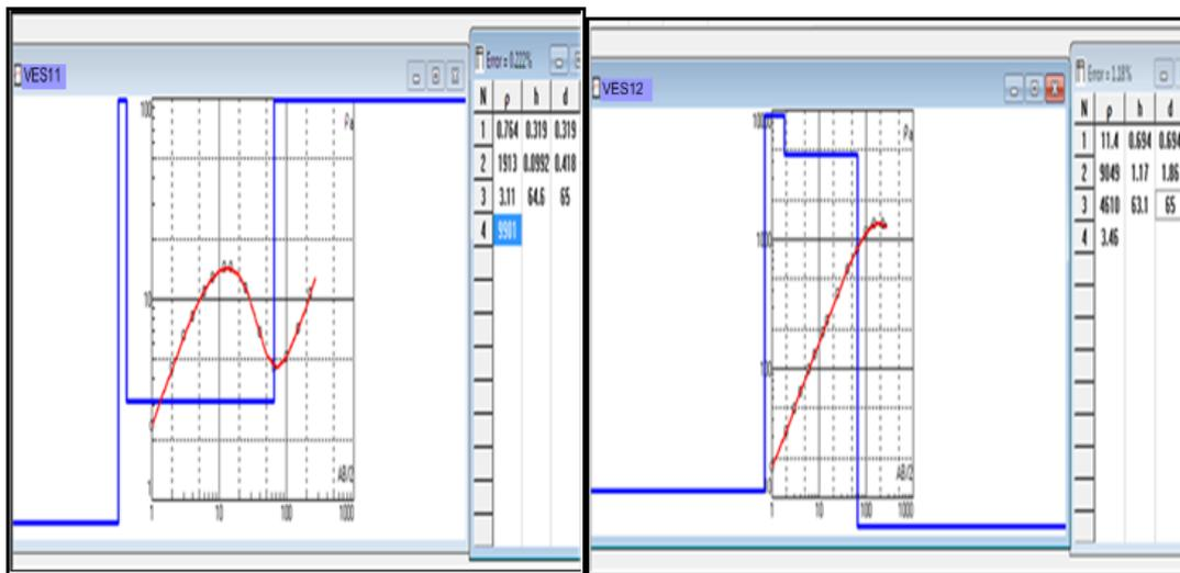
Figure 4(L): Geo-electric model & layer parameters for VES 12 (KQ curve type) Figure 4 (K): Geo-electric model & layer parameters for VES 11 (KH curve type)
