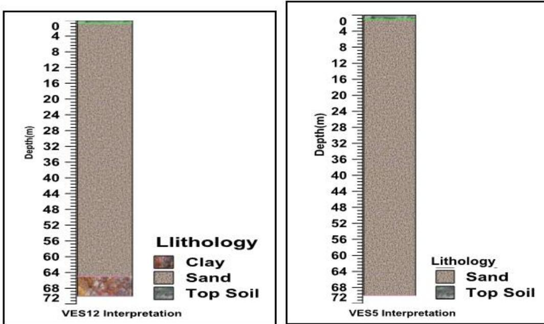
Figure 7: 1-D Geologic section of the subsurface for VES profile 12. Showing an unconfined aquifer within the second layer sand unit.
