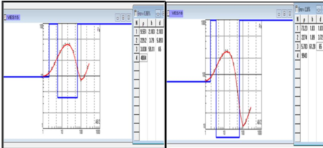
Figure 4 (O): Geo-electric model & layer parameters for VES 15 (KH curve type) Figure 4 (P): Geo-electric model & layer parameters for VES 16 (KH curve type).
