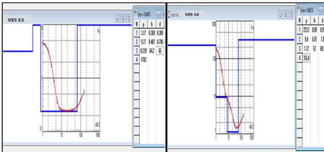
Figure 4 (N) : Geo-electric model & layer parameters for VES 14 (QH curve type) Figure 4 (M): Geo-electric model & layer parameters for VES 13 (KH curve type)
