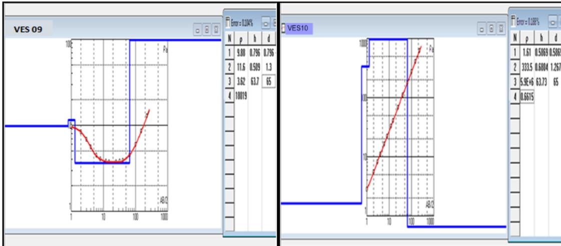
Figure 4 (J) : Geo-electric model & layer parameters for VES 10 (KQ curve type) Figure 4 (I): Geo-electric model & layer parameters for VES 9 (KH curve type).
