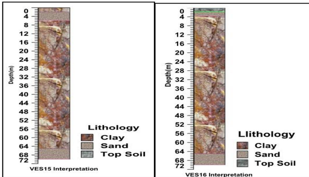
Figure 9: 1-D Geologic section of the subsurface for VES profile 15. Showing a Confined aquifer within the second and fourth layers.
