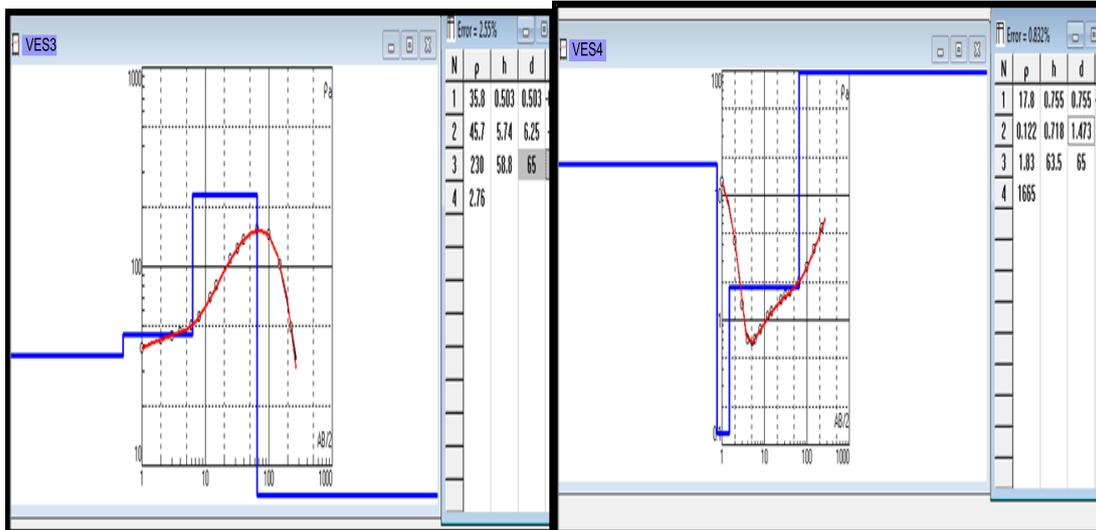
Figure 4 (D): Geo-electric model &layer parameters for VES 4(HK curve type).Figure 4(c): Geo-electric model &layer parameters for VES 3 (KA curve type).
