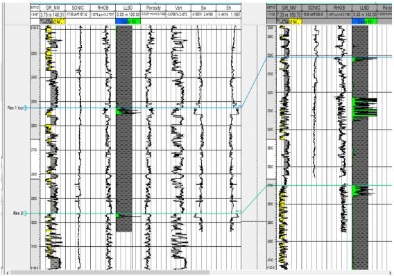
Figure 6: Porosity, shale volume, water saturation and hydrocarbon
