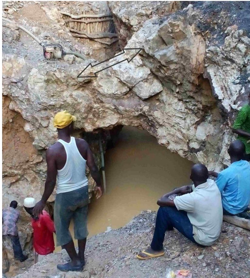
Fig 3. Azara Baryte Vein 17 (Note: Water level in pit and poor overpass which is already failing)
