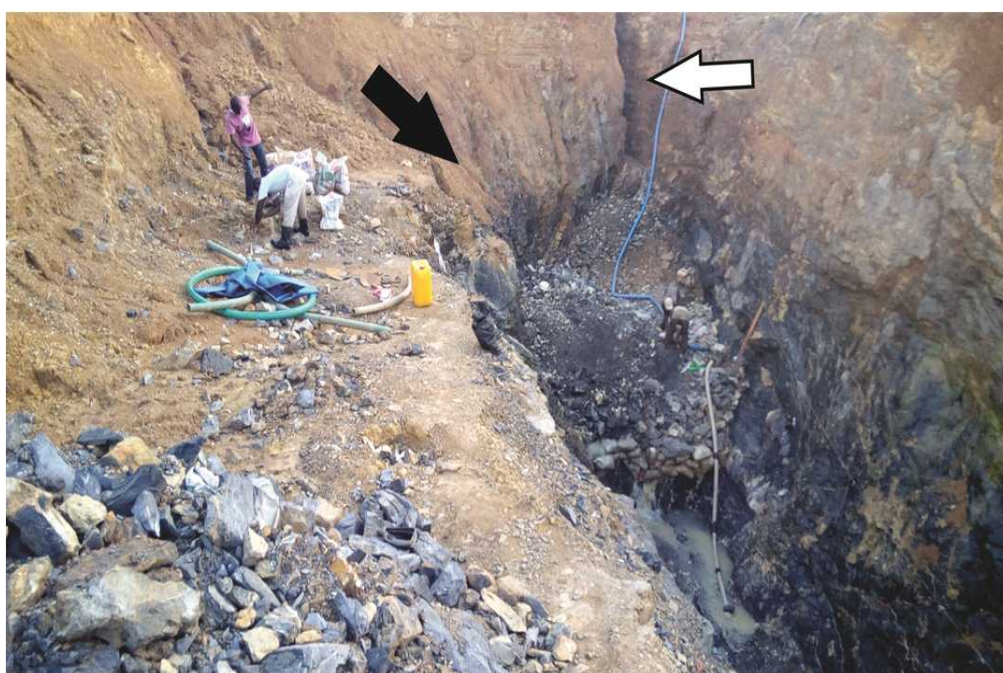
Fig 7. Typical mine in the Benue Trough with poor benching (Note: Dark arrow showing failed overburden with the lighter arrow showing cuts made by surface run-offs which pour into the mine)
