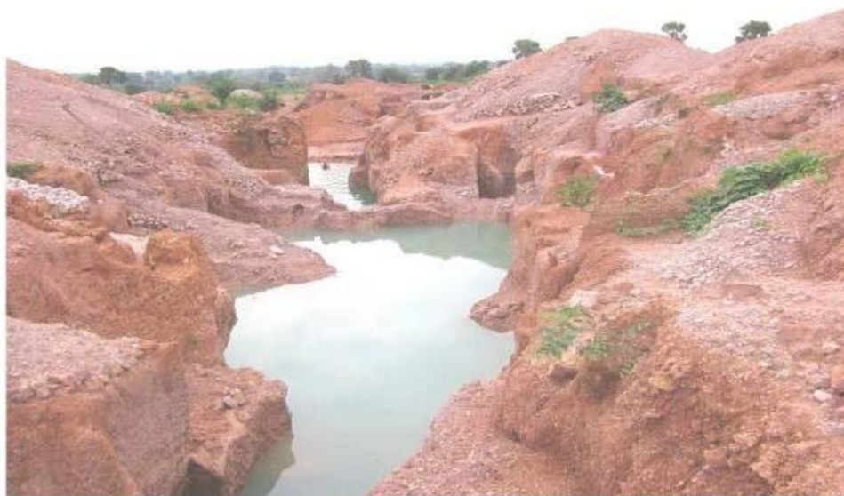
Fig 4. The Gabu Osina Baryte Vein in the Lower Benue Trough showing flooding peculiar to deposits across the trough (Oden, 2012)
