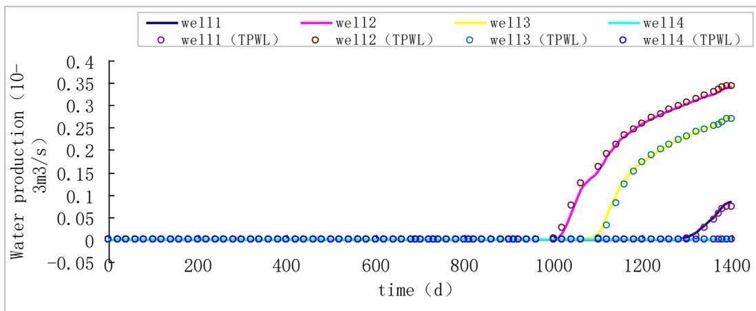
**Fig. 6** Water production contrast of four production wells (prediction process)
