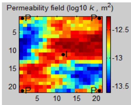
Fig.1 Permeability distribution of reservoir model
