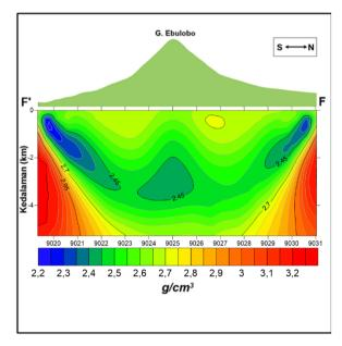
Figure 11. Modeling of the F-F' incision. Subsurface
