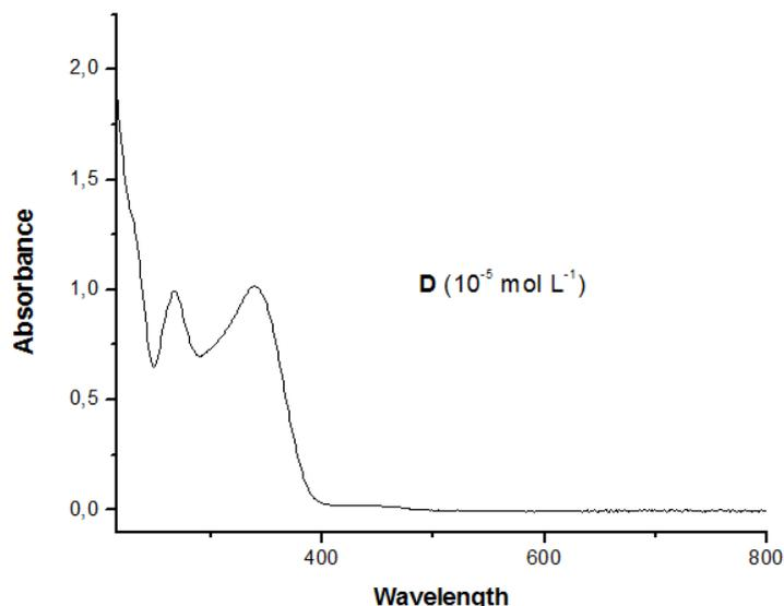
**Figure 3.** Spectra of complex-1 (A), complex-4 (B and C), and 3-*hmp* (D); A, B and D in methanol and C in DMSO. The spectra show MLCT, *d-d*,  $n \rightarrow \pi$ ,  $\pi \rightarrow \pi^*$  transitions and saturation of the detector in A, B and C below 500 nm.
