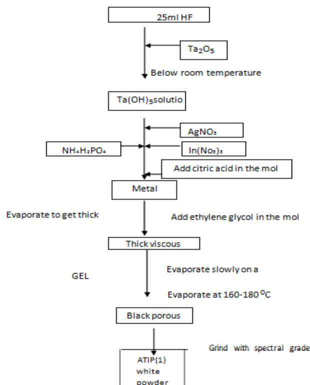
Fig.1 Flow chart of sol gel preparation procedure of ATP (1)
