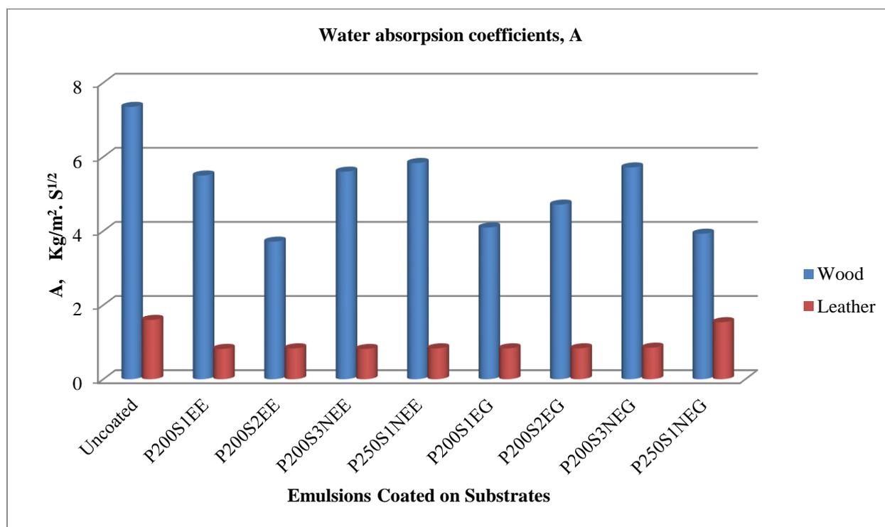
**Figure 1.** Water Absorption Coefficients of Substrates
