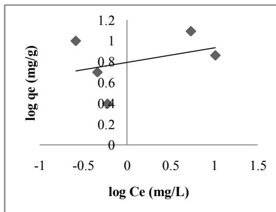
**Fig.5:** Freundlich isotherm for the adsorption of  $Pb^{2+}$  by native pulverized locust beans hull, pH7 at  $30 \pm 2^\circ C$ .
