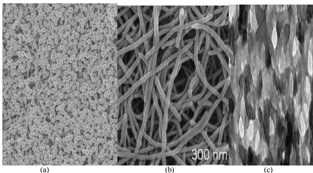
Figure 2: Different carbon nanostructures made by high-temperature catalysis, mimicking natural coalification however in a controlled technological environment: a) carbon nanoparticles for printing or reinforcement; b) carbon nanorods as texture modifier or conductance additive; c) sponge like carbon for water binding and ion exchange
