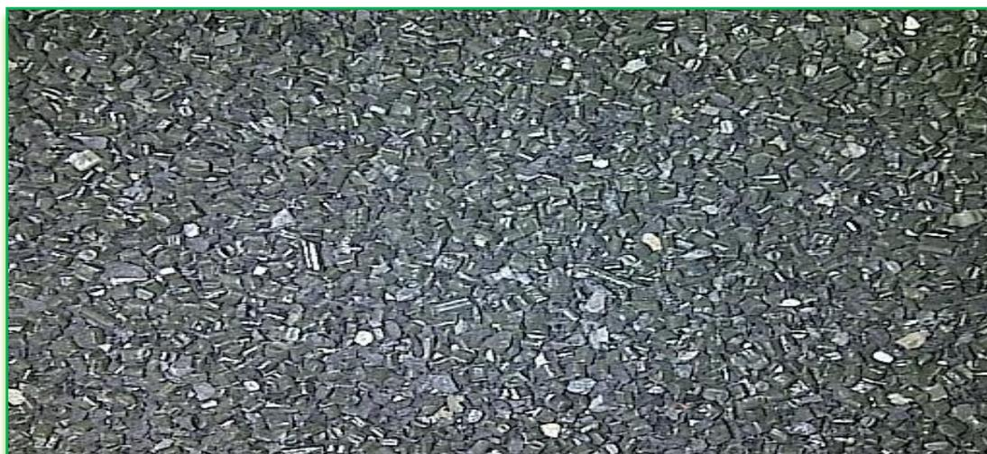
Plate I: Granular Activated carbon before remediation
