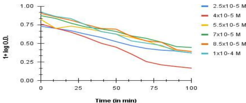
**Figure 10: Photodegradation of TB on Co<sub>3</sub>BaNiO<sub>6</sub> at different Concentrations of Dye (M)**
