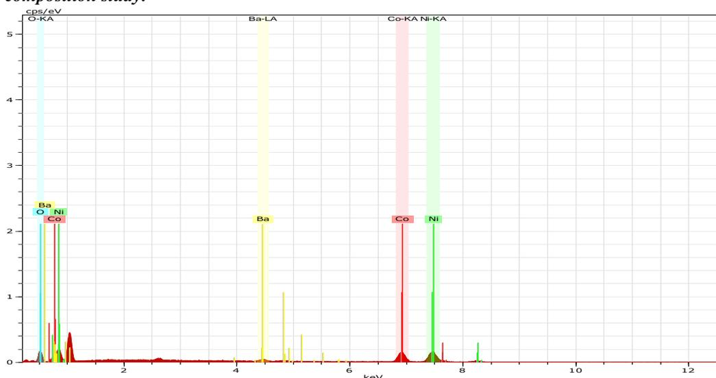
**Figure 1: EDS spectra of Co<sub>3</sub>BaNiO<sub>6</sub>**
