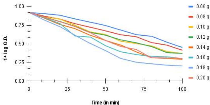
**Figure 9: Photodegradation of TB on Co<sub>3</sub>BaNiO<sub>6</sub> at different photocatalyst Dosage (g)**
