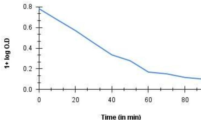
**Figure7: Photo Catalytic activity of Co<sub>3</sub>NiBaO<sub>6</sub>for degradation of TB**
