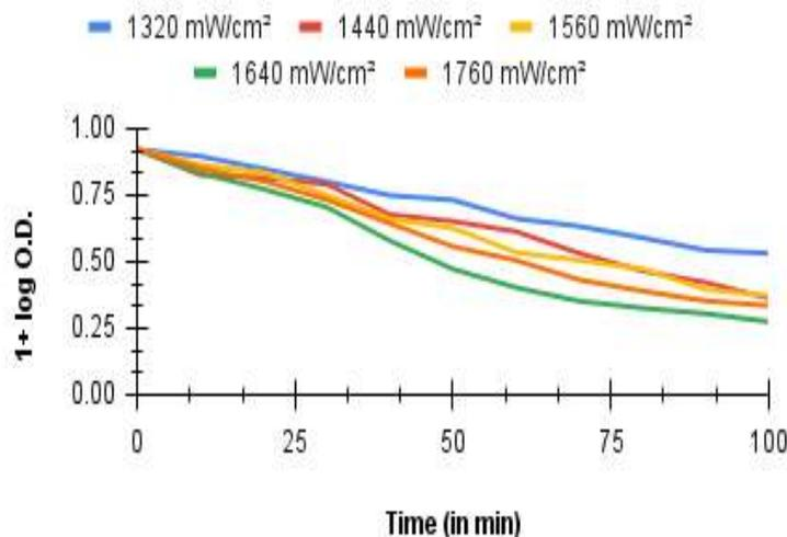
Figure 11: Photodegradation of TB on Co<sub>3</sub>BaNiO<sub>6</sub> at different Intensities of Light (in mW/cm<sup>2</sup>)
