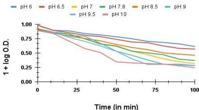
**Figure 8: Photodegradation of TB on Co<sub>3</sub>BaNiO<sub>6</sub>at different pH**
