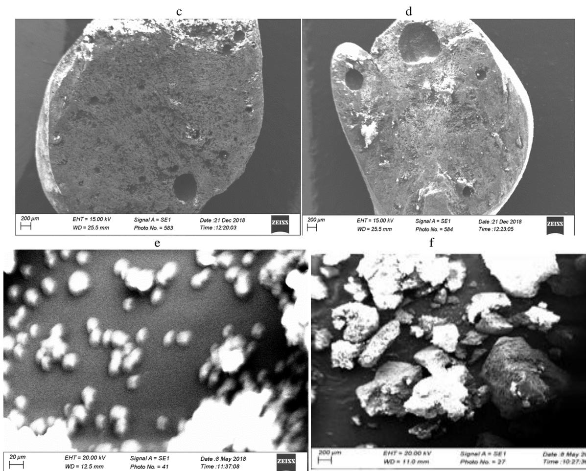
Fig. 3: (a) Photograph of starch beads and SEM micrograph showing (b) external morphology starch; (c) cross-section of dichlorvos-loaded starch and d diazinon-loaded starch; (e) internal morphology of dichlorvos-loaded starch and (f) diazinon-loaded starch.
