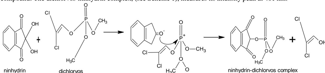
**Scheme 1:** A possible reaction of ninhydrin with 2,2-dichlorovinyl dimethyl phosphate (dichlorvos) to form dimethyl phosphate-ninhydrin complex
