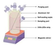
Figure no 3. Photocatalytic Reactor
