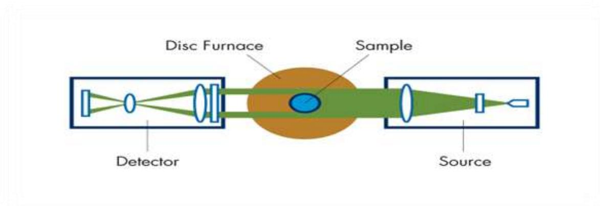
Fig 6.2: Working diagram of optical dilatometer DIL806
