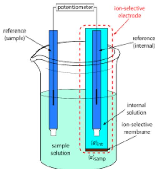
Figure 1. Potentiometric system in thermostated vessel
