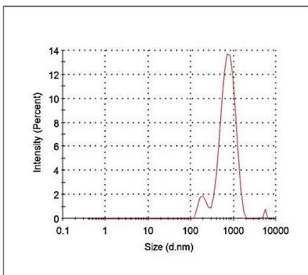
**Figure 4** Graph of particles size distribution by intensity of ZnO nanoparticles produced with LABS
