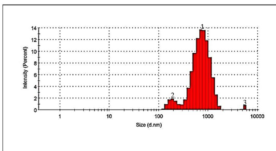
Figure 3 Size distributions by intensity of ZnO nanoparticles with LABS
