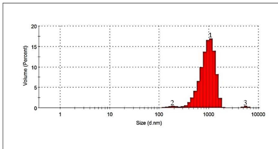
Figure 2 Size distribution by volume of LABS – capped ZnO nanoparticles
