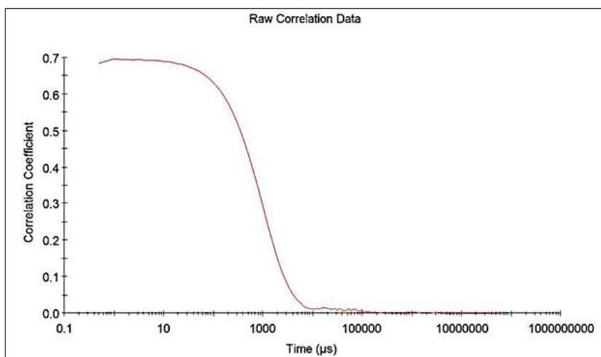
Figure 7 Correlogram for the cumulants for the ZnO nanoparticles
