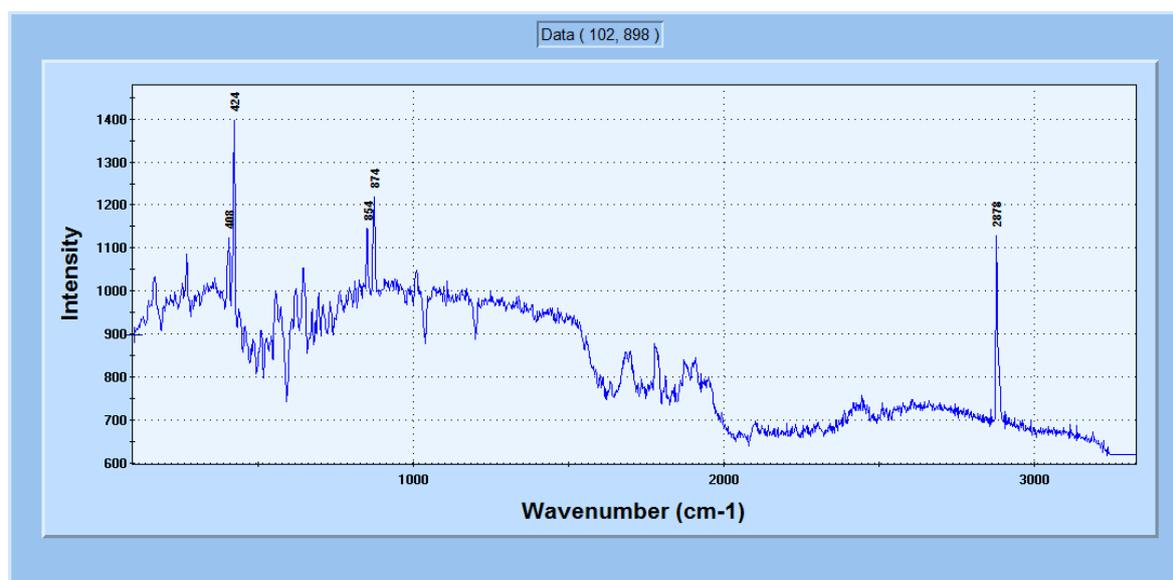
**Figure 1** Raman spectrum of ZnO nanoparticles produced with LABS.
