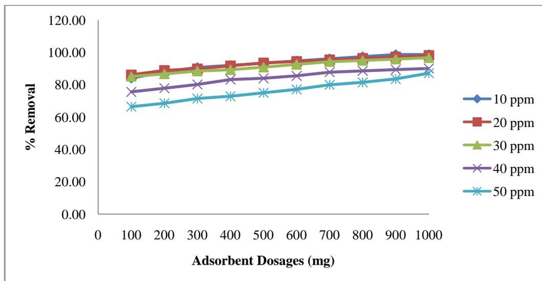
Fig.2: Effect of adsorbent dosages on the adsorption of Malachite green onto CPFAC.
