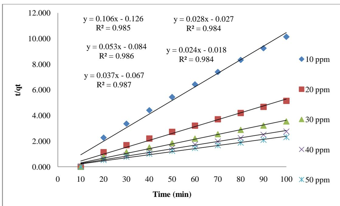
Fig.8: Pseudo- second order Kinetics for the adsorption of Malachite green onto prepared activated carbon at 30°C
