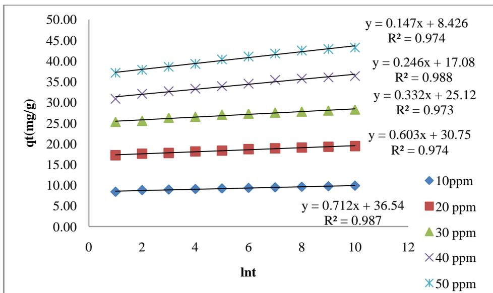
Fig.10: Elovich model for the adsorption of Malachite green onto prepared activated carbon at 30°C.
