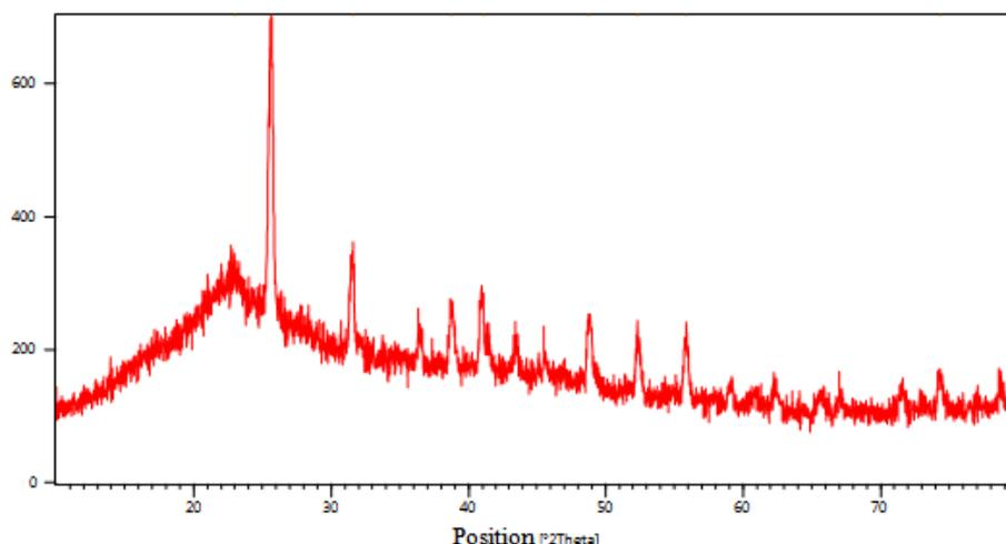
**Fig.6:** XRD pattern for prepared activated carbon
