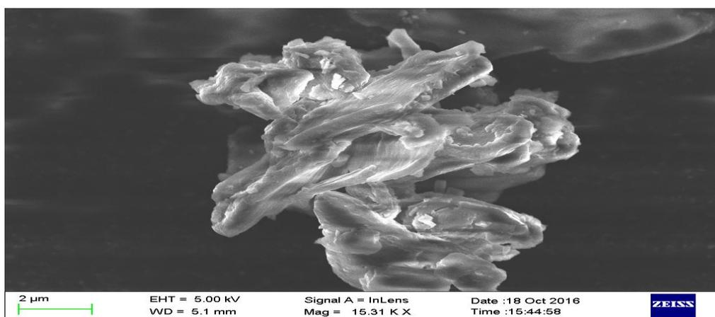
Fig.5: SEM image of activated carbon treated with Sulphuric acid
