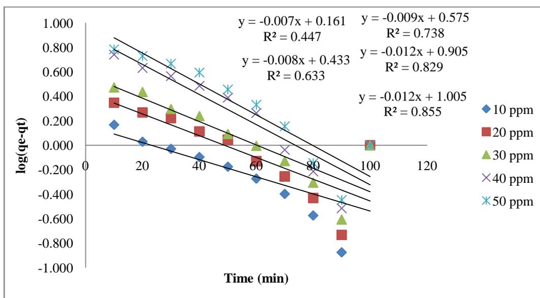
**Fig.7:** Pseudo-first order kinetics for adsorption of Malachite green onto prepared activated carbon at 30°C
