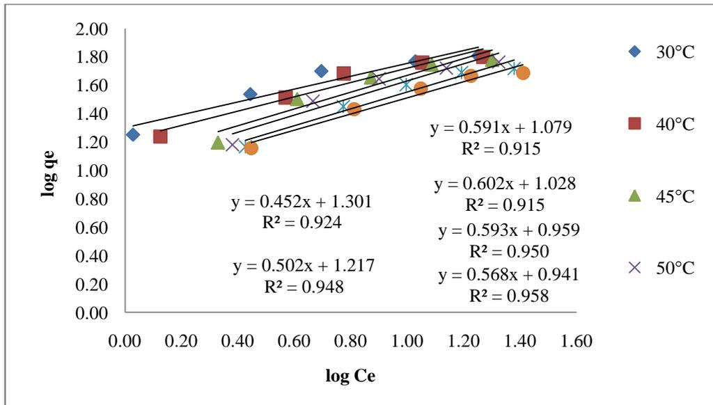
Fig.12: Freundlich isotherm for the adsorption of Malachite green onto prepared activated carbon.
