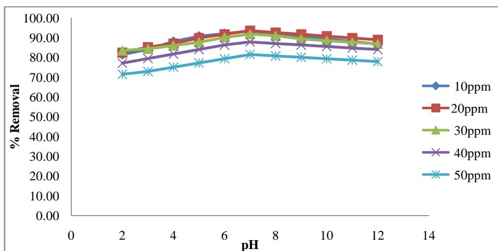
Fig.3: Effect of pH on the adsorption of Malachite green onto CPFAC.
