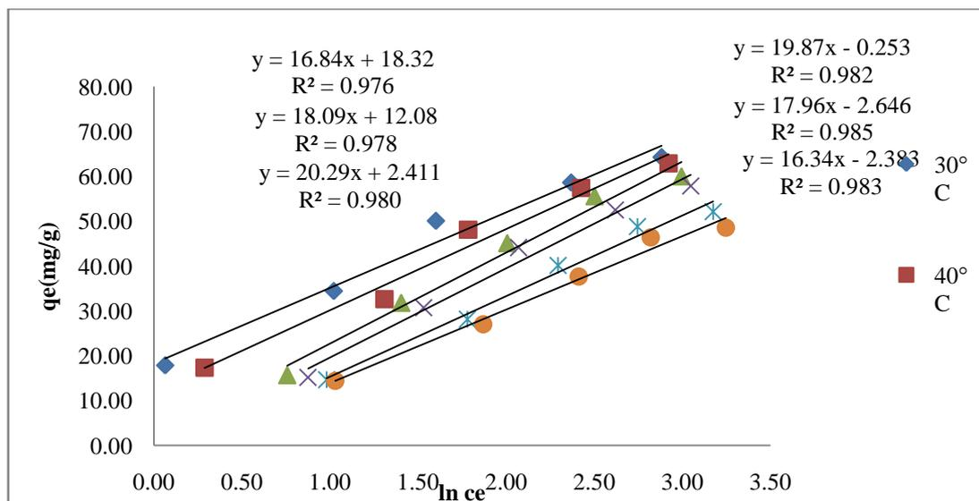
**Fig.13:** Tempkin isotherm for the adsorption of Malachite green onto prepared activated carbon.
