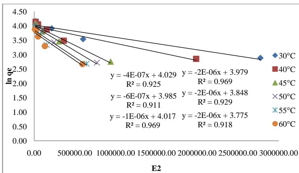
Fig.14: Dubinin -Radushkevich isotherm model for the adsorption of Malachite green onto prepared activated carbon.
