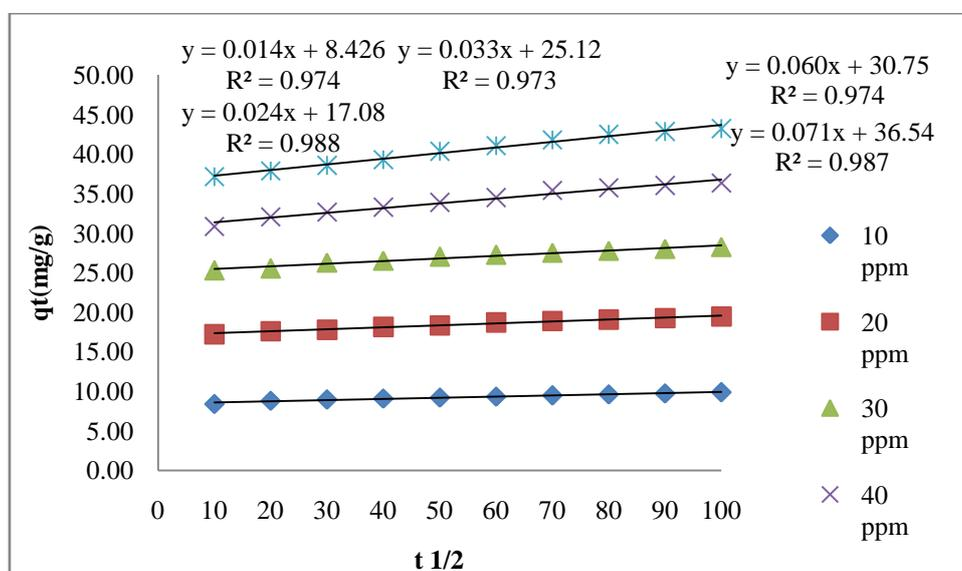
Fig.9: Intra particle diffusion for the adsorption of Malachite green onto prepared activated carbon at 30°C
