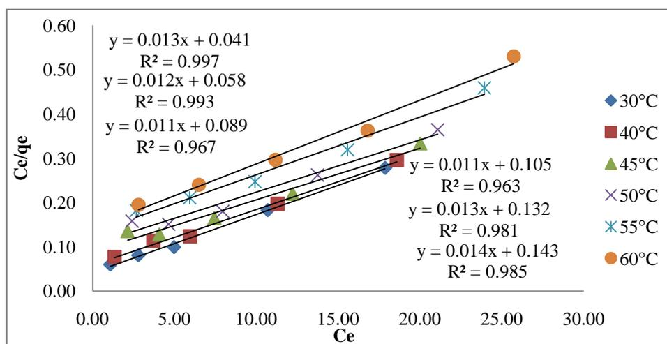
Fig.11: Langmuir isotherm for the adsorption of Malachite green onto prepared activated carbon.
