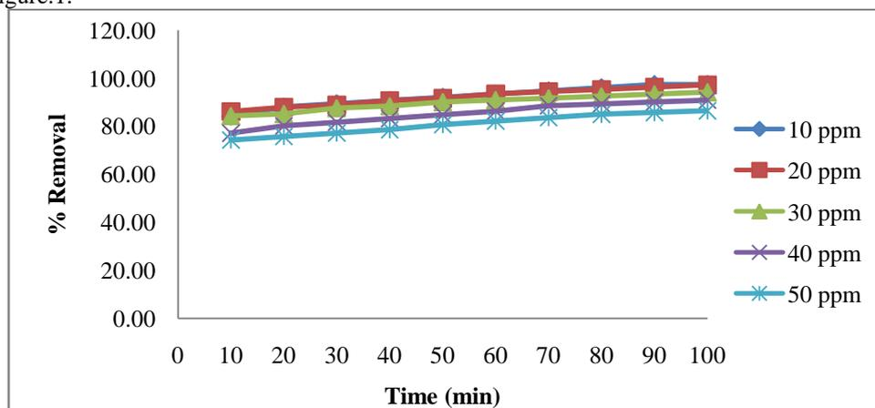
Fig.1: Effect of initial concentrations on the adsorption of Malachite green onto CPFAC.
