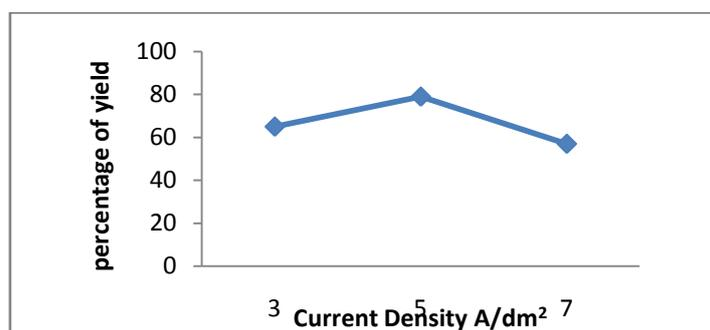
**Effect of current density using Graphite electrode in 1- Butanol**
