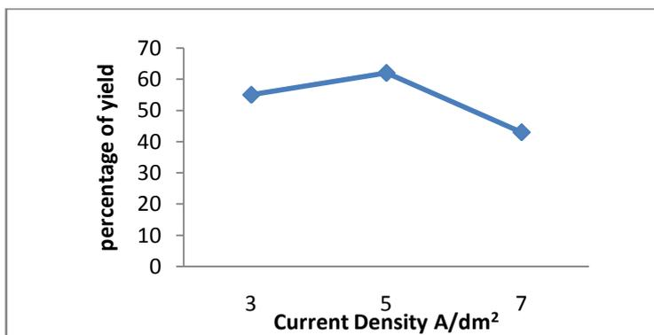
**Effect of current density using Platinum electrode in Acetonitrile**
