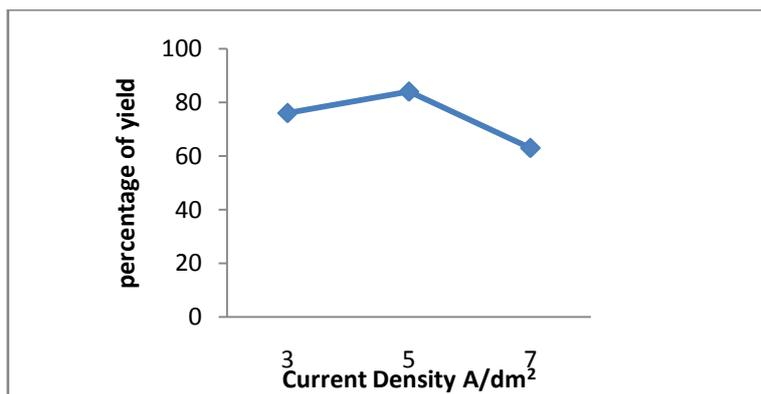
**Effect of current density using Graphite electrode in Dichloro Methane**
