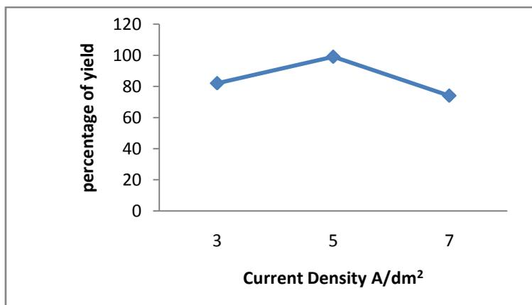
**Effect of current density using Platinum electrode in Dichloro Methane**
