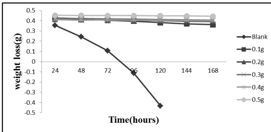
Fig. 2: Variation of Log ( $W_t - \Delta W$ ) with time for mild steel in 1M H<sub>2</sub>SO<sub>4</sub> at different concentrations of extracts.
