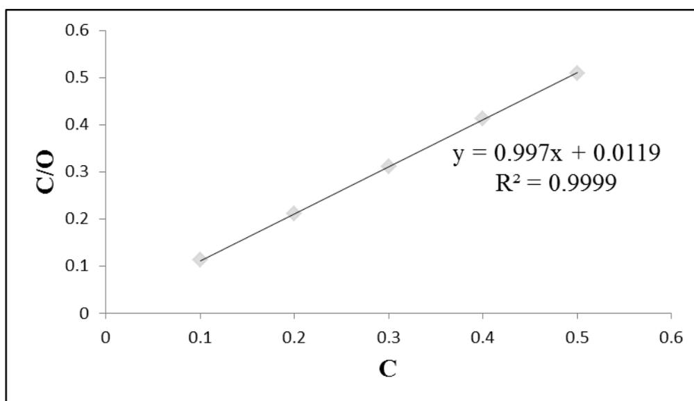
Fig. 4: Langmuir adsorption isotherm [c/e] plot versus concentration [c] for the inhibition of mild steel in 1M H<sub>2</sub>SO<sub>4</sub> solution
