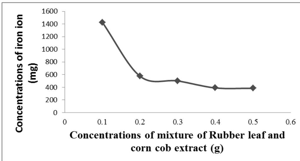
Fig. 5: Variations in concentrations of Iron ions ( $Fe^{2+}$ ,  $Fe^{3+}$ ) in 1M  $H_2SO_4$  acid solution from AAS.
