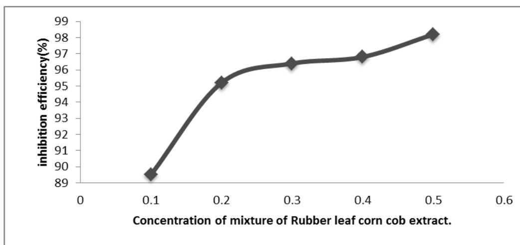
Fig. 3: Variation of inhibition efficiency with concentrations of mixture of Rubber leaf corn cob extract.
