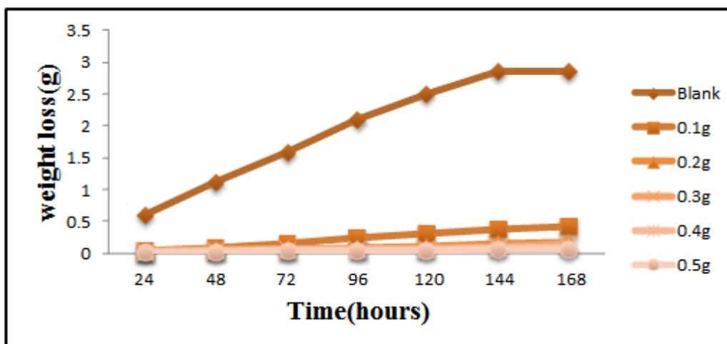
**Fig. 1:** Variation of weight loss with time for mild steel in 1M  $H_2SO_4$  at different concentrations of extracts.
