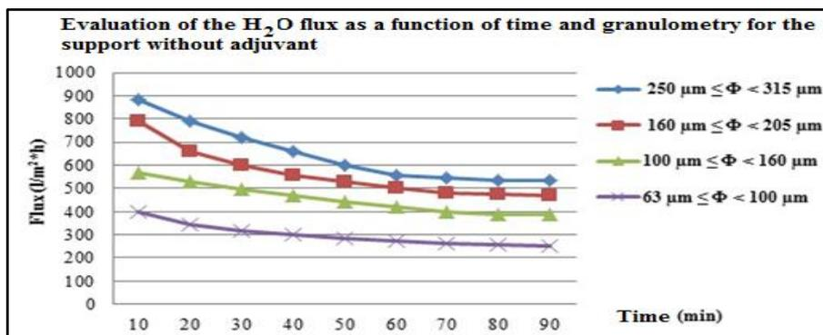
**Fig 2:** Flow through the support (AS) with different granulometry
