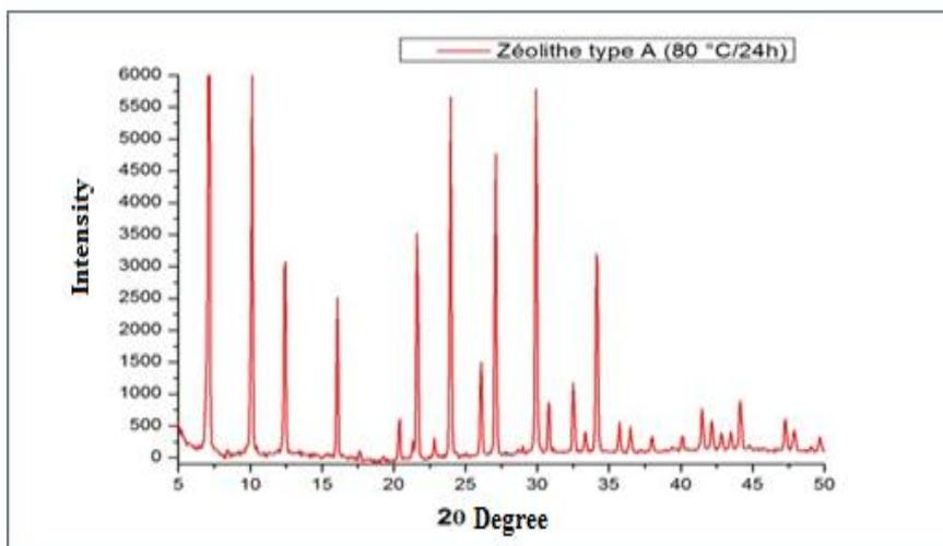
**Fig 8:** XRD of zeolitic type A ( $T = 80^{\circ}\text{C} / 24\text{h}$ )
