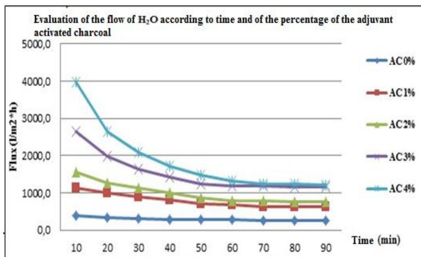
**Fig3:** Flow through the various supports AC.
