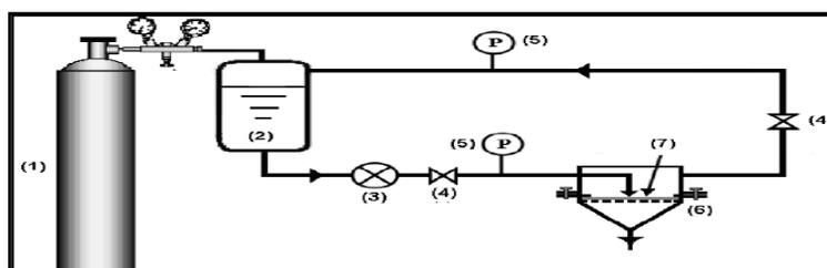
**Fig 1:** Diagram of the pilot of filtration: (1) nitrogenBottle (2)Water tank (3)circulating pump(4) valves(5) manometers (6)Modulates membrane (7) membrane.
