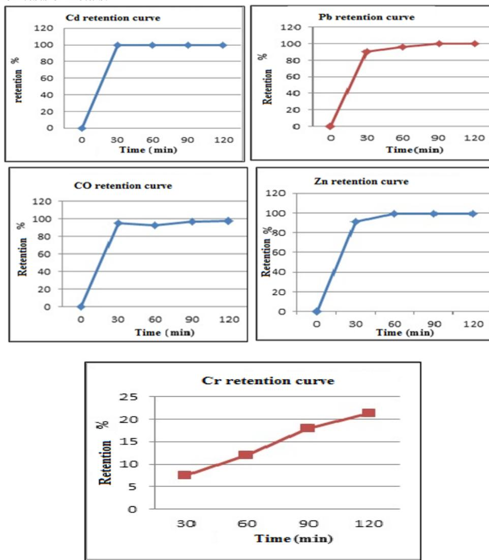
**Figure 10 :** Metal retention curves on ACZ-80 membrane.
