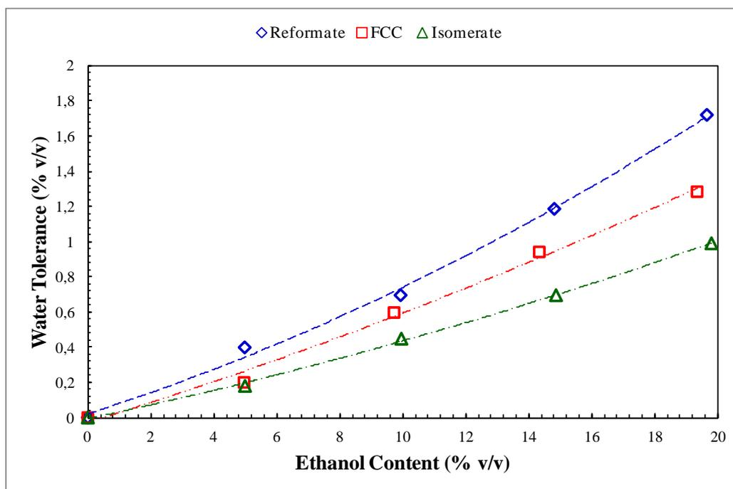
**Figure 1:** Water tolerance of refinery fractions
