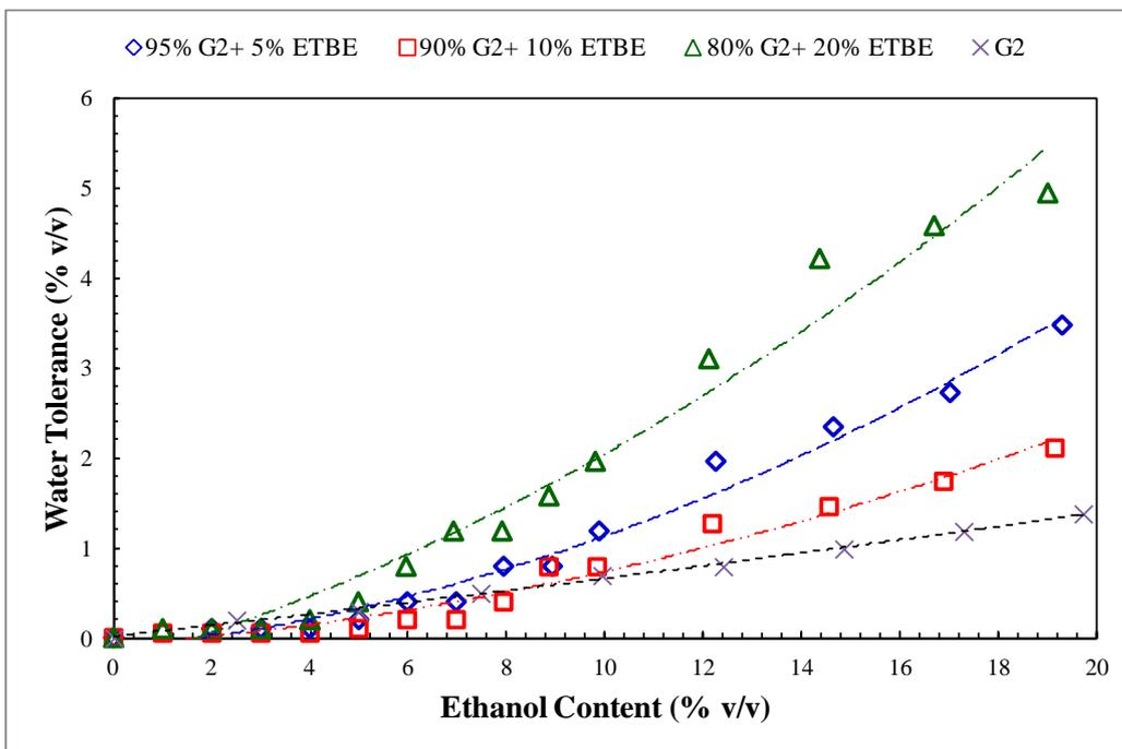
Figure 7: Water tolerance of G2 gasoline
