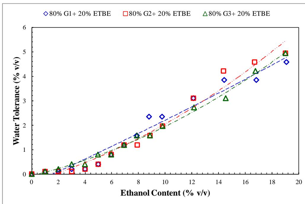
**Figure 5:** Water tolerance of gasolines with 20%v/v ETBE addition
