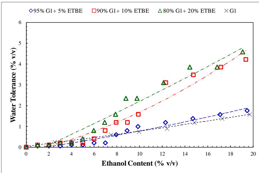
Figure 6: Water tolerance of G1 gasoline
