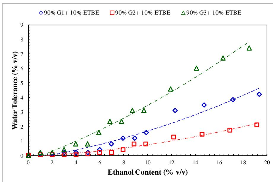
Figure 4: Water tolerance of gasolines with 10%v/v ETBE addition
