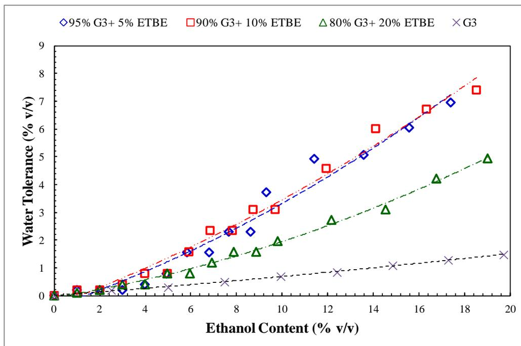
Figure 8: Water tolerance of G3 gasoline
