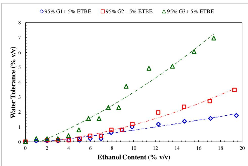
**Figure 3:** Water tolerance of gasolines with 5% v/v ETBE addition
