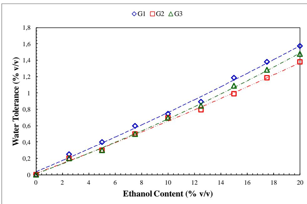
**Figure 2:** Water tolerance of G1, G2, G3 gasolines
